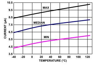
FIGURE 21. SUPPLY CURRENT DISABLED vs TEMPERATURE V<sub>+</sub>, V<sub>-</sub> = ±2.5V
