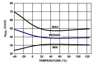
FIGURE 33. A<sub>VOL</sub> vs TEMPERATURE, R<sub>L</sub> = 1k V<sub>+</sub>, V<sub>-</sub> =  $\pm 2.5$ V, V<sub>O</sub> = -2V TO +2V
