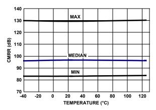
FIGURE 34. CMRR vs TEMPERATURE, V<sub>CM</sub> = +2.5V TO -2.5V, V<sub>+</sub>, V<sub>-</sub> =  $\pm 2.5V$
