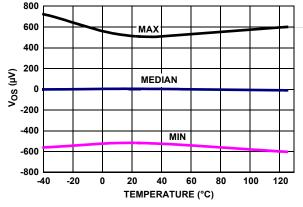
FIGURE 25.  $V_{OS}$  (SOT PKG) vs TEMPERATURE  $V_{IN}$  = 0V, V<sub>+</sub>, V<sub>2</sub> = ±2.5V
