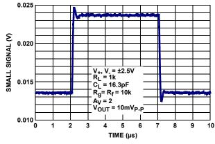
FIGURE 16. SMALL SIGNAL STEP RESPONSE
