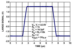
FIGURE 15. LARGE SIGNAL STEP RESPONSE
