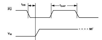
\*MI in the AC timing diagram refers to the minimum incremental change in the wiper voltage.
