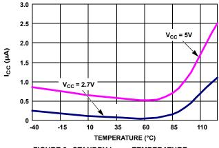
FIGURE 2. STANDBY I<sub>CC</sub> vs TEMPERATURE
