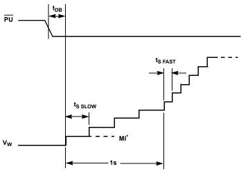
\*MI in the AC timing diagram refers to the minimum incremental change in the wiper voltage.
