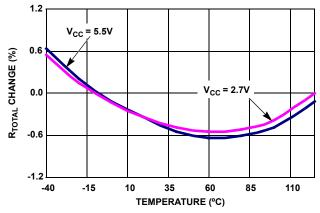
FIGURE 9. END TO END R<sub>TOTAL</sub> % CHANGE vs TEMPERATURE
