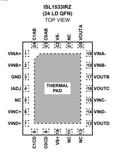
THERMAL PAD TO BE CONNECTED TO GND
