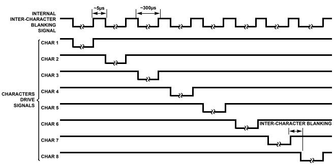
FIGURE 3. DISPLAY CHARACTERS MULTIPLEX TIMING DIAGRAM
