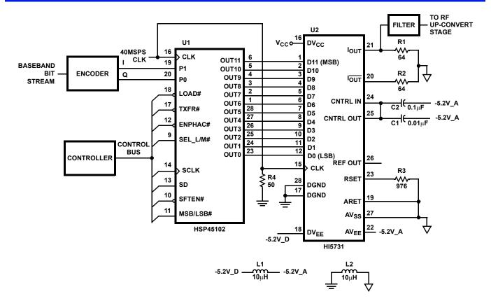
FIGURE 29. PSK MODULATOR USING THE HI5731 AND THE HSP45102 12-BIT NCO
