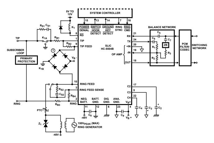
FIGURE 1. TYPICAL LINE CIRCUIT APPLICATION WITH THE MONOLITHIC SLIC
