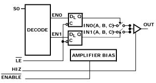
A LOGIC HIGH ON LE WILL LATCH THE LAST SO STATE. THI<u>S LOGIC</u> STATE IS PRESERVED WHEN CYCLING HIZ OR ENABLE FUNCTIONS.
