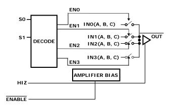
FIGURE 2. FUNCTIONAL DIAGRAM EL4342
