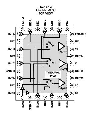
THERMAL PAD INTERNALLY CONNECTED TO V-. PAD MUST BE TIED TO V-NIC = NO INTERNAL CONNECTION
