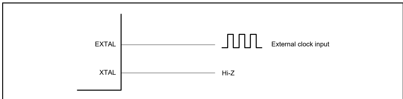
Figure 9.5 Equivalent circuit for external clock
