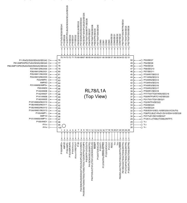
Caution Connect the REGC pin to VSS pin via a capacitor (0.47 to 1  $\mu$ F).
