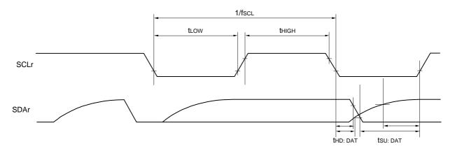
Remark 1.  $Rb[\Omega]$ : Communication line (SDAr) pull-up resistance, Cb[F]: Communication line (SDAr, SCLr) load capacitance
