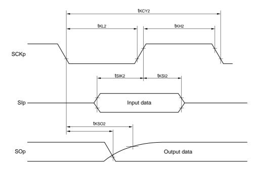
Simplified SPI (CSI) mode serial transfer timing (slave mode) (during communication at different potential) (When DAPmn = 0 and CKPmn = 1, or DAPmn = 1 and CKPmn = 0.)
