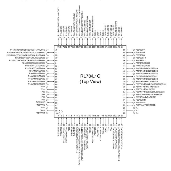
Caution Connect the REGC pin to Vss pin via a capacitor (0.47 to 1  $\mu$ F).
