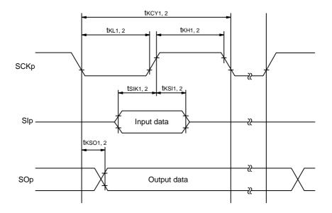
Simplified SPI (CSI) mode serial transfer timing (during communication at same potential)
