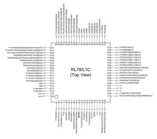
Caution Connect the REGC pin to Vss pin via a capacitor (0.47 to 1  $\mu$ F).
