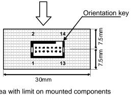
Area with limit on mounted components (heights must be no greater than 5 mm)
