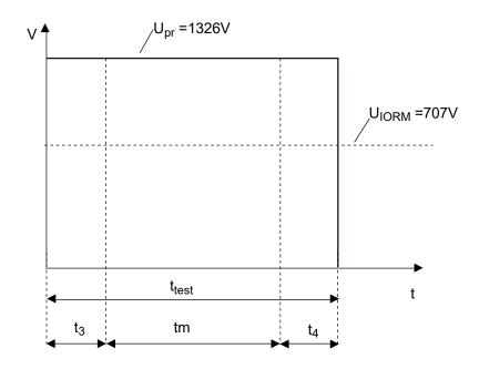
$t_3$ ,  $t_4$  = 0.1 sec  $t_{m(PARTIAL\ DISCHARGE)}$ = 1.0 sec  $t_{test}$  = 1.2 sec
