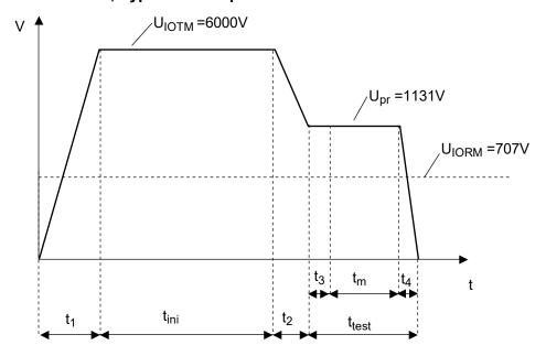
$t_1, t_2 = 1 \text{ to } 10 \text{ sec}$  $t_3, t_4 = 1 \text{ sec}$
