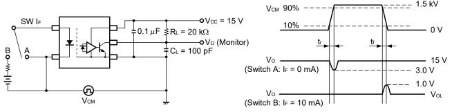
C∟ includes probe and stray wiring capacitance.
