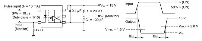
CL includes probe and stray wiring capacitance.
