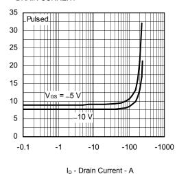
$R_{\text{DS}(on)}$  - Drain to Source On-state Resistance -  $m\Omega$
