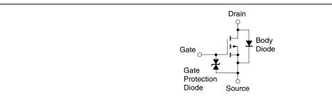
**Remark** The diode connected between the gate and source of the transistor serves as a protector against ESD. When this device actually used, an additional protection circuit is externally required if a voltage exceeding the rated voltage may be applied to this device.
