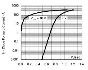
$V_{\text{F(S-D)}}$  - Source to Drain Voltage - V
