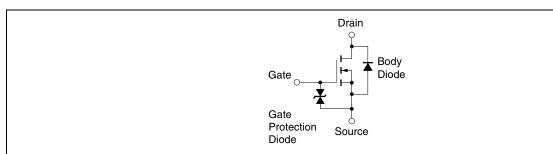
**Remark** The diode connected between the gate and source of the transistor serves as a protector against ESD. When this device actually used, an additional protection circuit is externally required if a voltage exceeding the rated voltage may be applied to this device.
