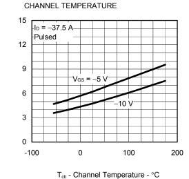
DRAIN TO SOURCE ON-STATE RESISTANCE vs.
