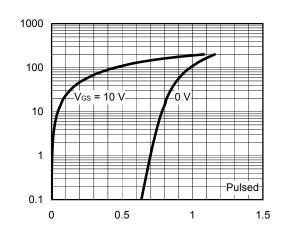
$V_{F(S\text{-}D)}$  - Source to Drain Voltage - V
