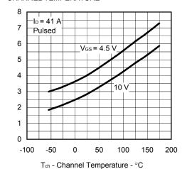
R<sub>DS(on)</sub> - Drain to Source On-state Resistance - mΩ
