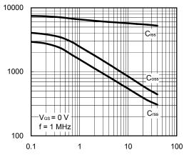
CAPACITANCE vs. DRAIN TO SOURCE VOLTAGE
