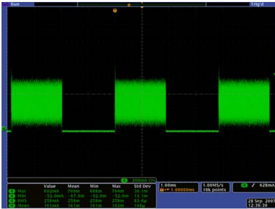
FIGURE 10. I L AT 50% PWM DIMMING (54LEDs, 20mA, V IN = 12V, L = 8.2μH)
