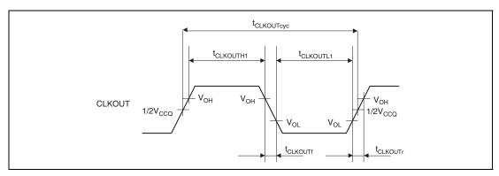
Figure 43.3 CLKOUT Clock Output Timing (1)
