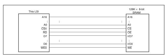
Figure 11.8 Example of 8-Bit Data-Width SRAM Connection
