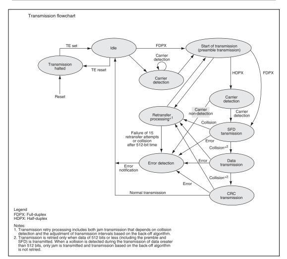
Figure 23.9 E-MAC Transmitter State Transitions
