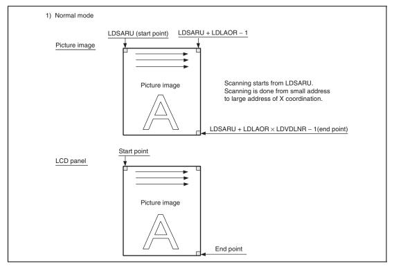
Figure 37.9 Operation for Hardware Rotation (Normal Mode)
