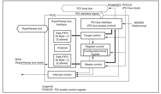
Figure 13.1 PCIC Block Diagram
