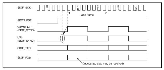
Figure 29.22 SIOF\_SYNC Output Timing in Master Mode 2 (Transfer Started)
