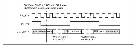
Figure 34.2 Philips Format (with no Padding)
