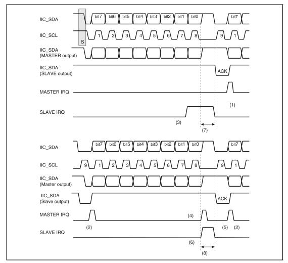
Figure 26.9 Data Transmit Mode Operation Timing
