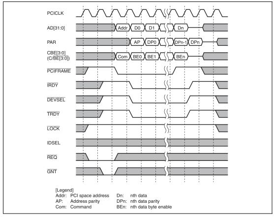
Figure 13.19 Master Write Cycle in Normal Mode (Burst)
