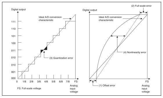
Figure 38.5 Definitions of A/D Conversion Accuracy
