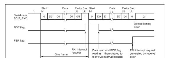
Figure 28.11 shows an example of the operation for reception in asynchronous mode.
