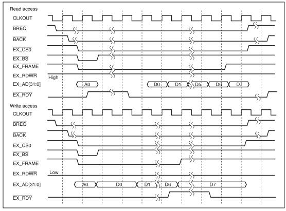
Figure 15.3 External CPU Access (Burst Access)
