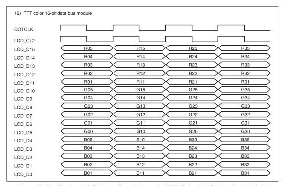
Figure 37.22 Clock and LCD Data Signal Example (TFT Color 16-Bit Data Bus Module)
