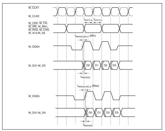
Figure 43.29 Read Timing of DDR-SDRAM (2 Burst Read)
