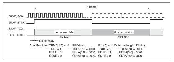
Figure 29.16 Transmit and Receive Timing (16-Bit Stereo Data (1))
