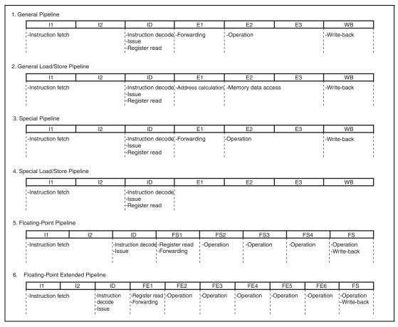
Figure 4.1 Basic Pipelines
