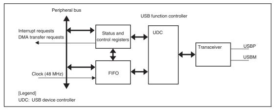
Figure 36.1 Block Diagram of USBF
