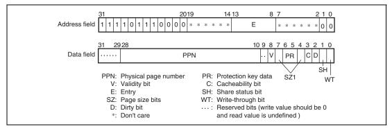
Figure 6.15 Memory-Mapped UTLB Data Array
