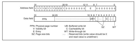
Figure 6.19 Memory-Mapped PMB Data Array
