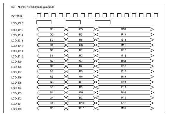
Figure 37.16 Clock and LCD Data Signal Example (STN Color 16-Bit Data Bus Module)
