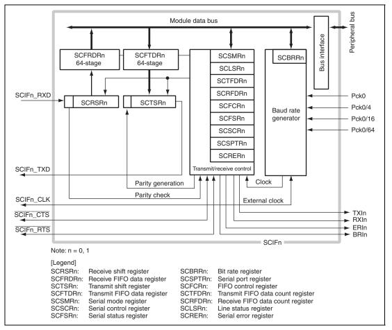
Figure 27.1 Block Diagram of SCIF
