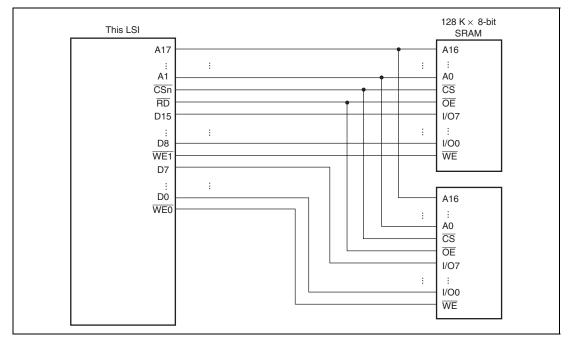
Figure 11.7 Example of 16-Bit Data-Width SRAM Connection
