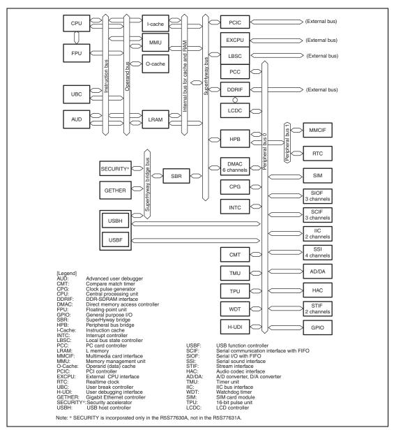
Figure 1.1 SH7763 Block Diagram
