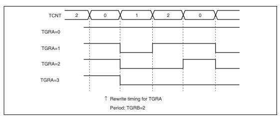
Figure 20.13 Examples of PWM Mode Operation (2)
