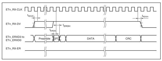
Figure 43.42 MII Receive Timing (normal operation)
