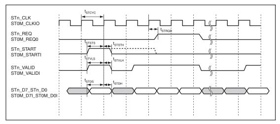
Figure 43.52 STIF Clock Valid Receive Timing
