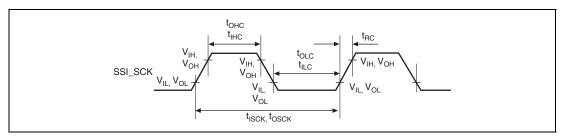
Figure 43.73 SSI Clock Input/Output Timing
