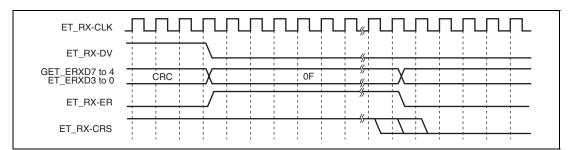
Figure 23.24 GMII/MII Fame Receive Timing (with Carrier Extension)
