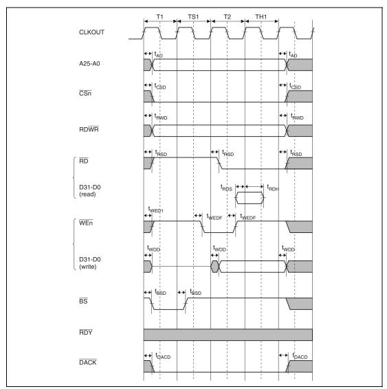
Figure 43.14 SRAM Bus Cycle: Basic Bus Cycle
