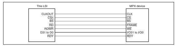
Figure 11.22 Example of 32-Bit Data Width MPX Connection
