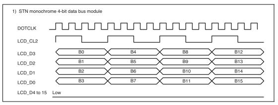
Figure 37.11 Clock and LCD Data Signal Example
