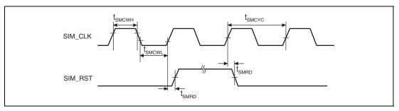
Figure 43.66 SIM Module Signal Timing
