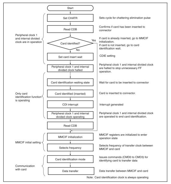
Figure 31.21 Operation Flow to Apply the Card Identification Function
