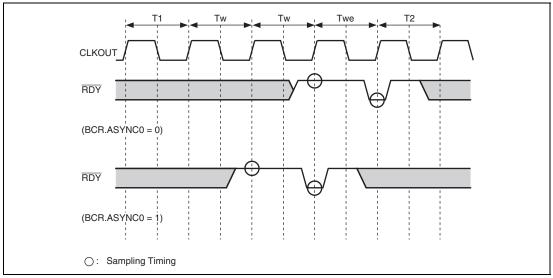
Figure 11.4 RDY Sampling Timings with ASYNCn Settings (Two Wait Cycles Inserted by CSnWCR.)
