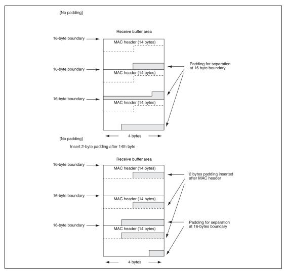
Figure 23.14 Padding Insertion in Receive Data
