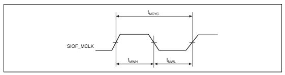
Figure 43.60 SIOF\_MCLK Input Timing
