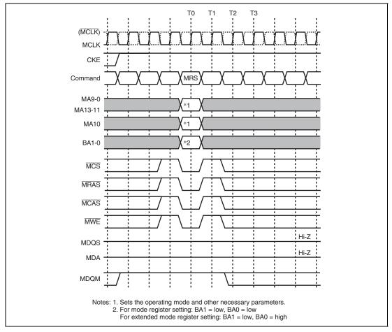
Figure 12.12 Basic DDRIF Timing (Mode Register Set (MRS))
