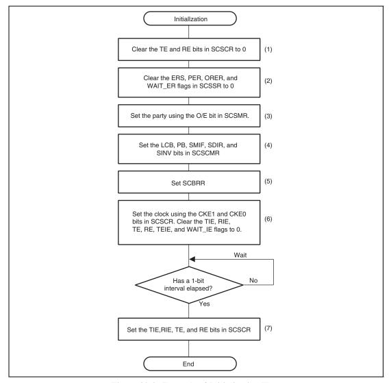
Figure 30.4 Example of Initialization Flow
