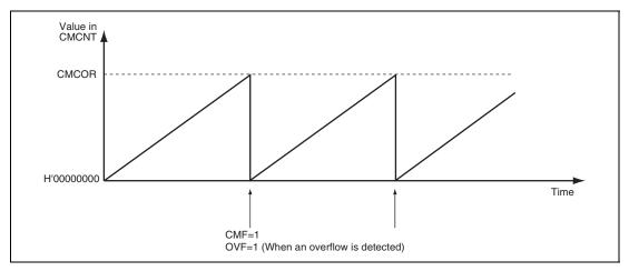
Figure 21.3 Counter Operation (Free-Running Operation)
