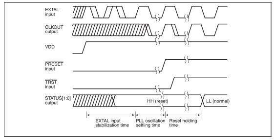
Figure 17.3 STATUS Output during Power-on
