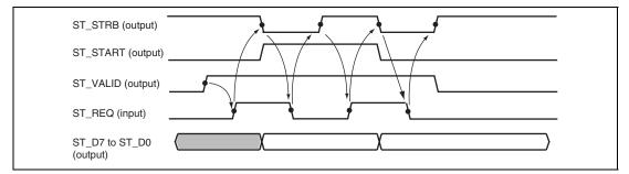
Figure 25.6 Strobe Transmission Timing
