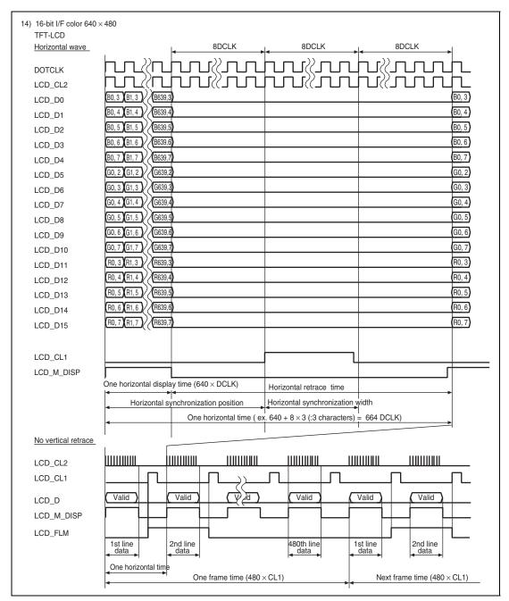
Figure 37.24 Clock and LCD Data Signal Example (16-Bit Interface Color 640 × 480)
