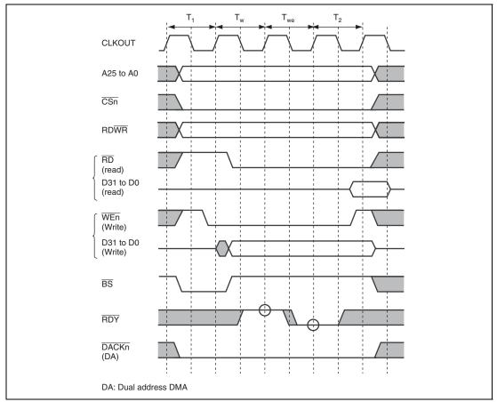
Figure 11.10 SRAM Interface Wait Cycle Timing (Wait Cycle Insertion by RDY Signal)
