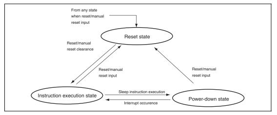
**Figure 2.8 Processing State Transitions**
