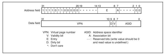
Figure 6.14 Memory-Mapped UTLB Address Array
