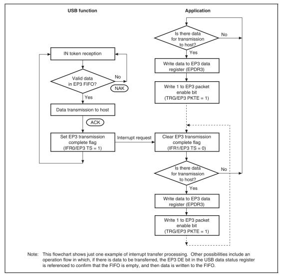
Figure 36.12 EP3 Interrupt-In Transfer Operation
