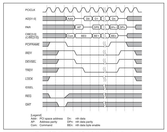
Figure 13.20 Master Read Cycle in Normal Mode (Burst)
