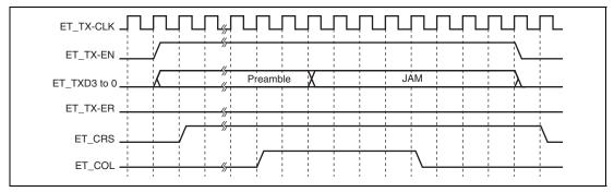
Figure 23.18 MII Frame Transmit Timing (Collision)
