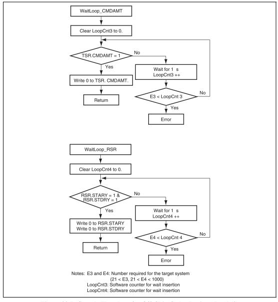
Figure 33.7 Sample Flowchart for Off-Chip Codec Register Read (3)
