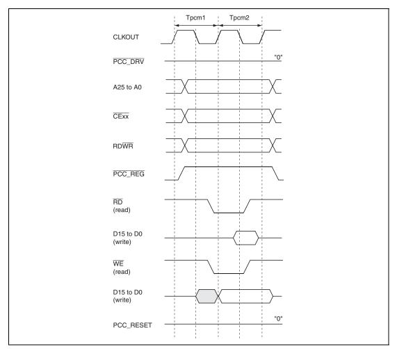
Figure 32.5 PCMCIA Memory Card Interface Basic Timing
