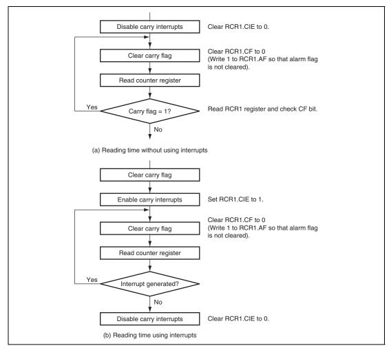
Figure 22.3 Examples of Time Reading Procedures
