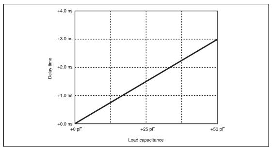
Figure 43.86 Load Capacitance - Delay Time
