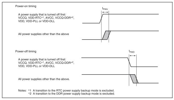
Figure 43.1 Power-On and Power-Off Timing
