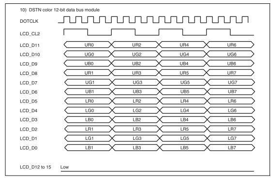
Figure 37.20 Clock and LCD Data Signal Example (DSTN Color 12-Bit Data Bus Module)
