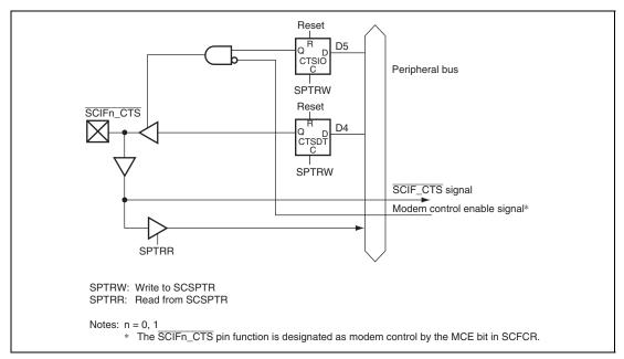
Figure 27.3  $\overline{\text{SCIFn}\_\text{CTS}}$  Pin (n = 0, 1)
