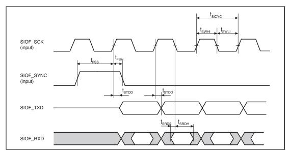
Figure 43.65 SIOF Transmission/Reception Timing (Slave Mode 1, Slave Mode 2)
