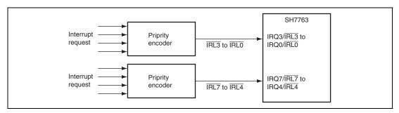
Figure 9.2 Example of IRL Interrupt Connection
