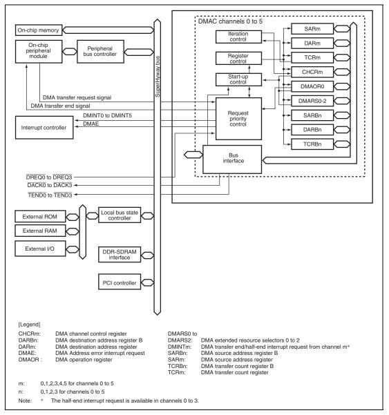
Figure 14.1 Block Diagram of DMAC
