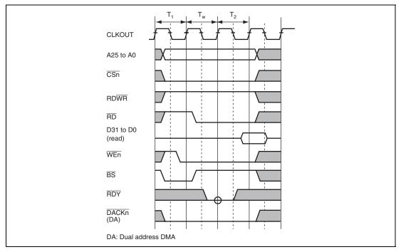
Figure 11.37 Byte-Control SRAM Basic Read Cycle (One Internal Wait Cycle)
