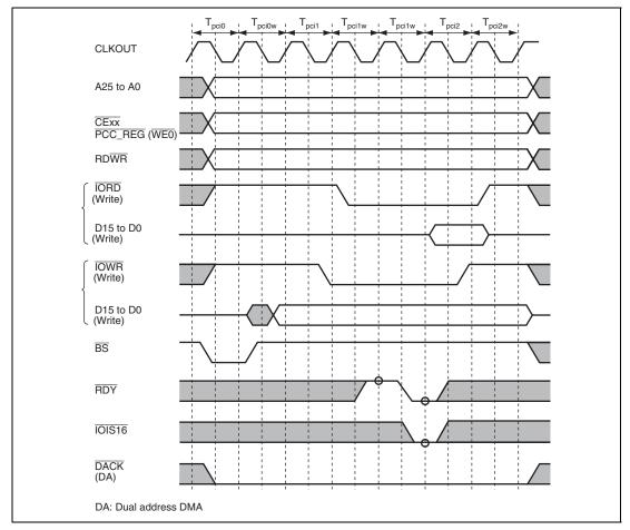
Figure 11.20 Wait Timing for PCMCIA I/O Card Interface
