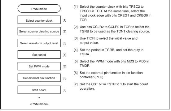
Figure 20.11 Example of PWM Mode Setting Procedure
