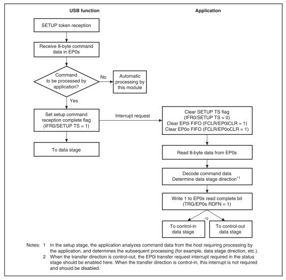
Figure 36.5 Setup Stage Operation
