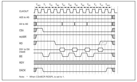
Figure 11.14 Burst ROM Wait Access Timing
