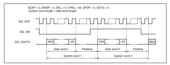
Figure 34.3 Philips Format (with Padding)
