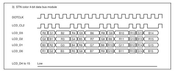
Figure 37.13 Clock and LCD Data Signal Example (STN Color 4-Bit Data Bus Module)
