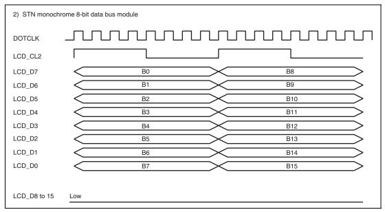
Figure 37.12 Clock and LCD Data Signal Example (STN Monochrome 8-Bit Data Bus Module)
