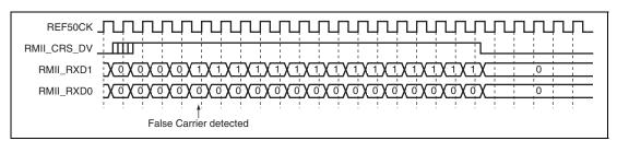
Figure 23.30 RMII Fame Receive Timing (100-Mbps Reception with Illegal Carrier **Detected**)
