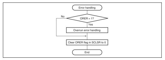
Figure 27.19 Sample Serial Reception Flowchart (2)
