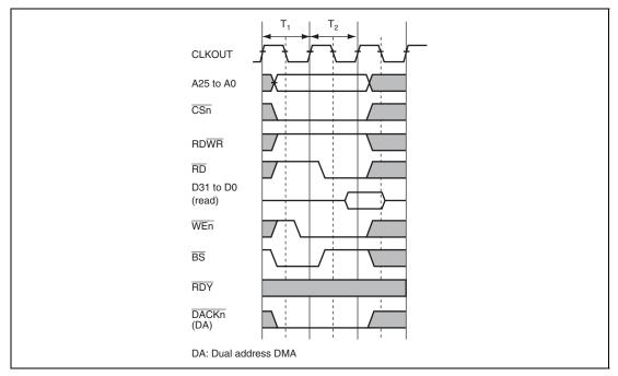
Figure 11.36 Byte-Control SRAM Basic Read Cycle (No Wait)
