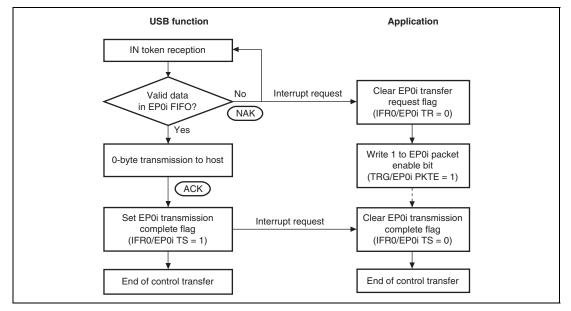
Figure 36.9 Status Stage (Control-Out) Operation
