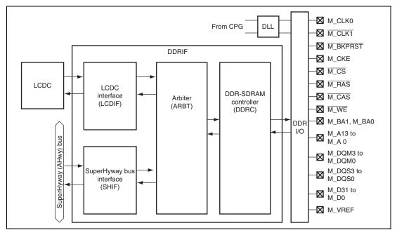
Figure 12.1 DDRIF Block Diagram
