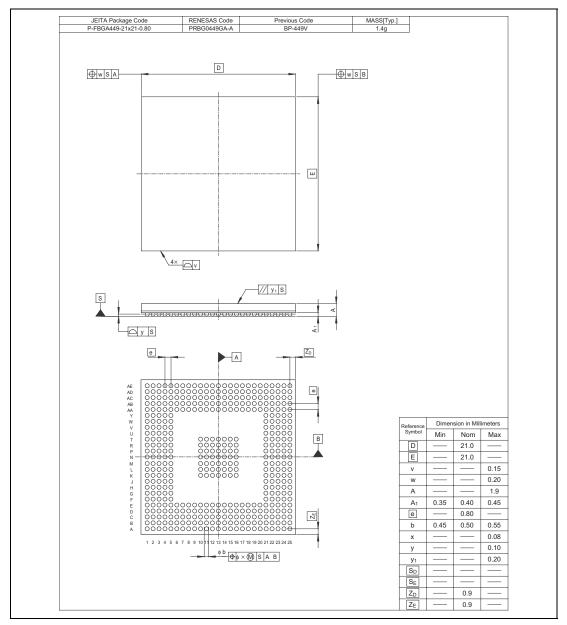
Figure D.1 Package Dimensions (449-Pin)
