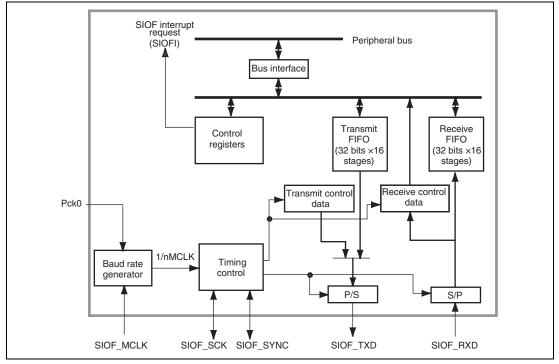
Figure 29.1 Block Diagram of SIOF
