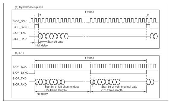
Figure 29.3 Serial Data Synchronization Timing
