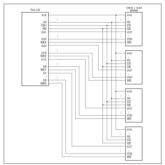
Figure 11.6 Example of 32-Bit Data-Width SRAM Connection
