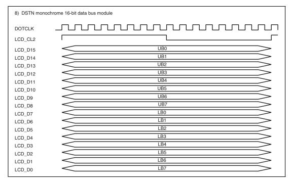
Figure 37.18 Clock and LCD Data Signal Example (DSTN Monochrome 16-Bit Data Bus Module)
