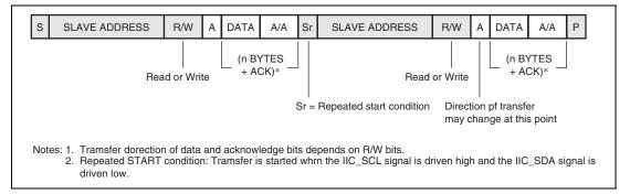
Figure 26.5 Combination Transfer Format of Master Transfer
