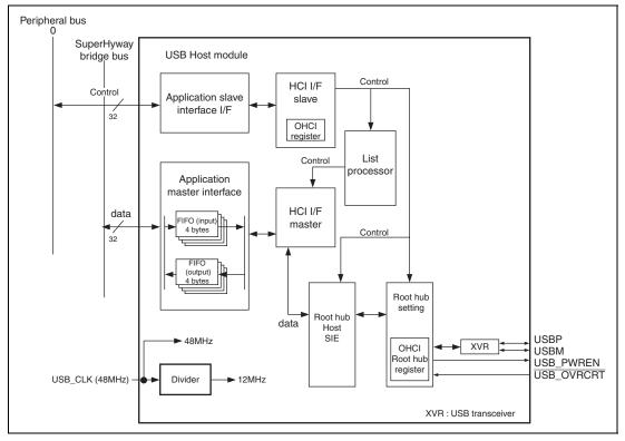
Figure 35.1 Block Diagram of USBH
