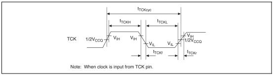
Figure 43.81 TCK Input Timing
