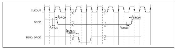
Figure 43.37 DREQ, TEND, and DACK Timing
