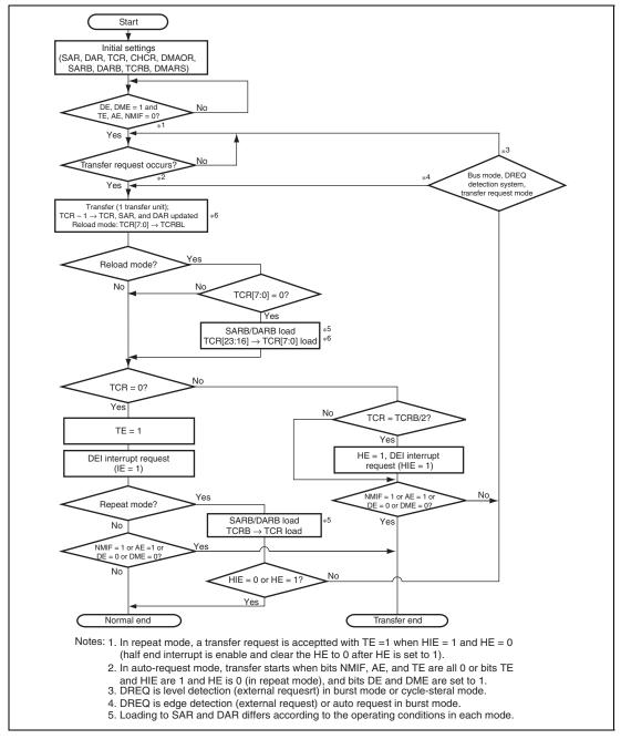
Figure 14.11 DMA Transfer Flowchart
