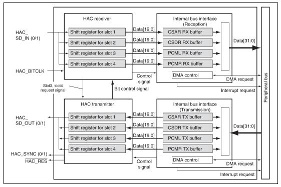
Figure 33.1 Block Diagram
