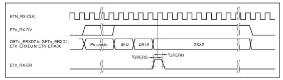
Figure 43.47 GMII Receive Timing (When an Error is Detected)
