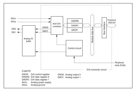
Figure 39.1 Block Diagram of D/A Converter
