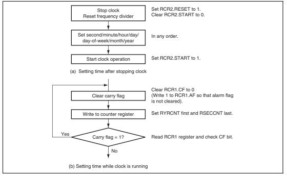
Figure 22.2 Examples of Time Setting Procedures
