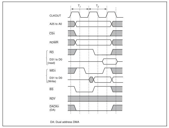
Figure 11.5 Basic Timing of SRAM Interface
