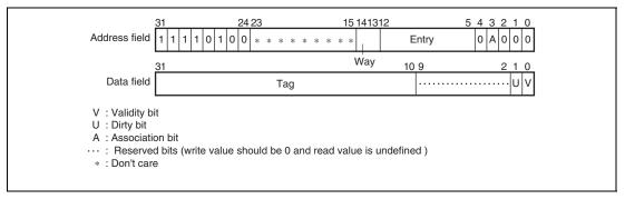
Figure 7.7 Memory-Mapped OC Address Array
