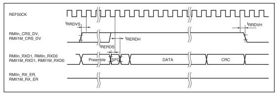
Figure 43.50 RMII Receive Timing (normal operation)
