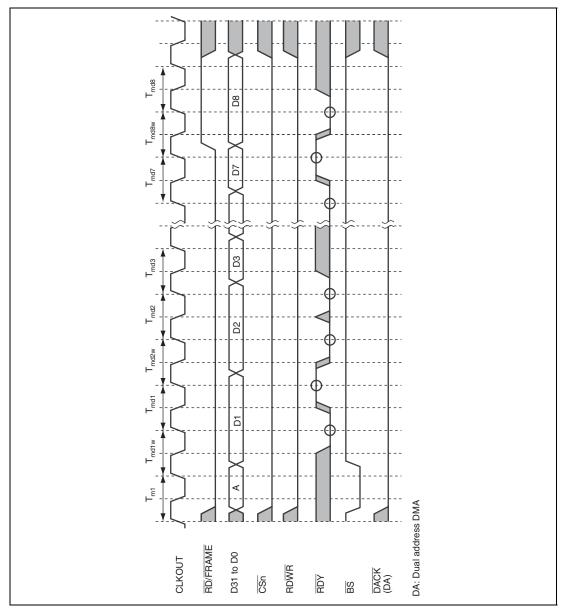
Figure 11.34 MPX Interface Timing 12 (Burst Write Cycle, IW = 1, External Wait Control, 32-Bit Bus Width, 32-Byte Data Transfer)
