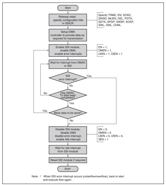
Figure 34.19 Transmission Using DMA Controller
