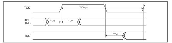
Figure 43.83 H-UDI Data Transfer Timing
