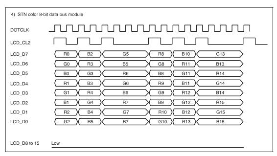
Figure 37.14 Clock and LCD Data Signal Example (STN Color 8-Bit Data Bus Module)
