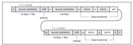
Figure 26.8 10-Bit Address Transmit/Receive Combined Format
