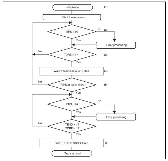
Figure 30.5 Example of Transmit Processing
