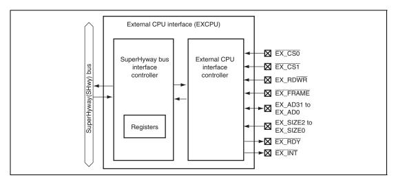
Figure 15.1 EXCPU Block Diagram
