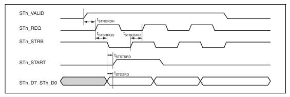
Figure 43.55 STIF Strobe Transmit Timing
