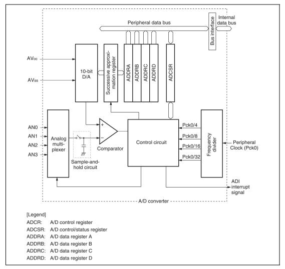
Figure 38.1 Block Diagram of A/D Converter
