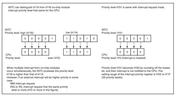
Figure 9.3 On-chip Module Interrupt Priority
