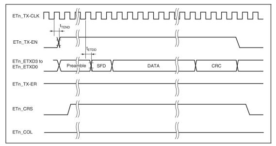
Figure 43.41 MII Transmit Timing (normal operation)
