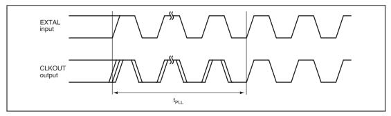
Figure 43.6 PLL Synchronization Settling Time
