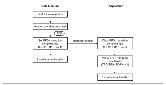
Figure 36.8 Status Stage (Control-In) Operation
