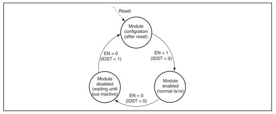
Figure 34.18 Transition Diagram between Operation Modes
