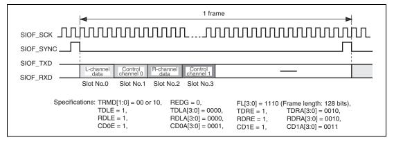
Figure 29.7 Control Data Interface (Slot Position)
