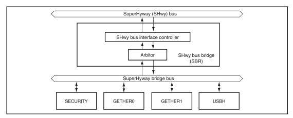
Figure 10.1 SBR Block Diagram
