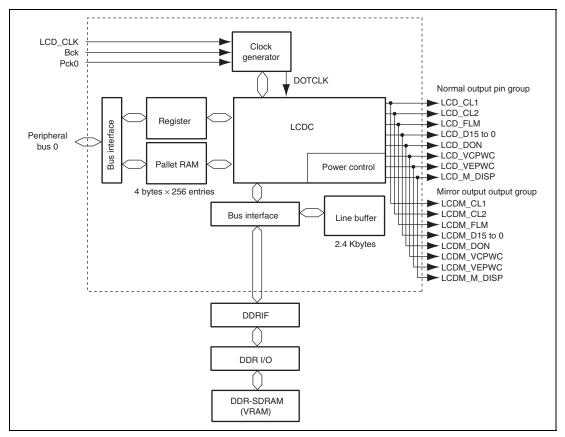
Figure 37.1 LCDC Block Diagram
