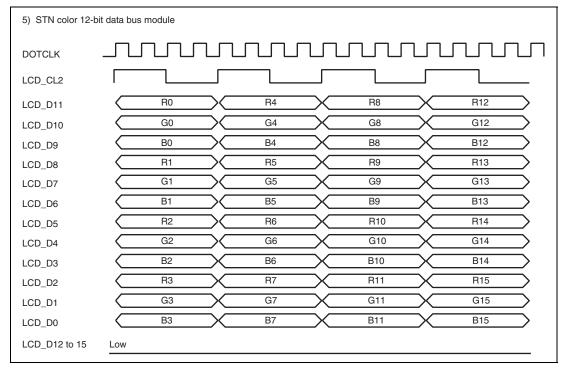
Figure 37.15 Clock and LCD Data Signal Example (STN Color 12-Bit Data Bus Module)
