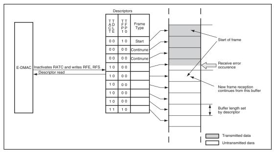
Figure 23.13 E-DMAC Operation after Receive Error
