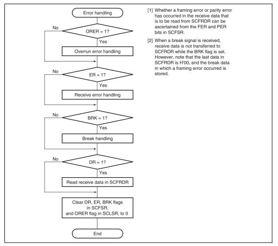
Figure 27.12 Sample Serial Reception Flowchart (2)
