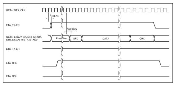
Figure 43.45 GMII Transmit Timing (normal operation)
