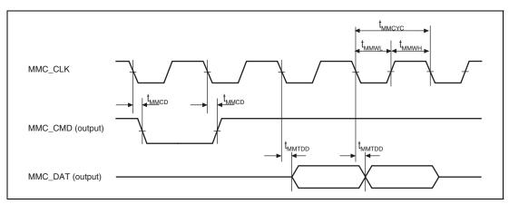
Figure 43.67 MMCIF Transmit Timing
