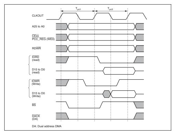
Figure 11.19 Basic Timing for PCMCIA I/O Card Interface
