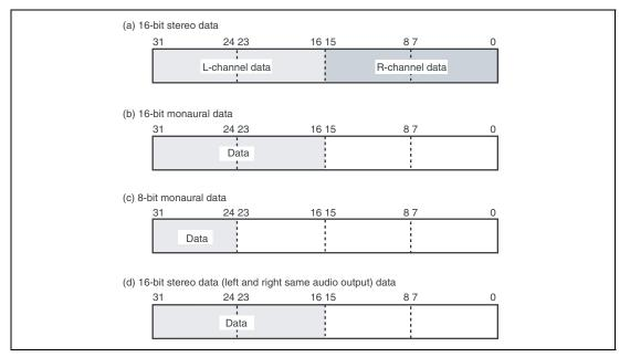
Figure 29.5 Transmit/Receive Data Bit Alignment
