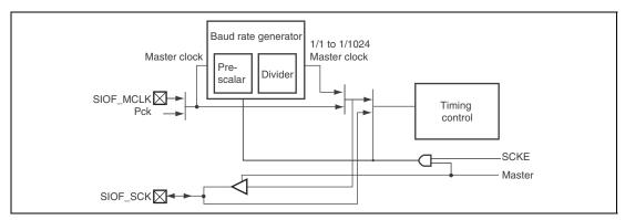
Figure 29.2 Serial Clock Supply
