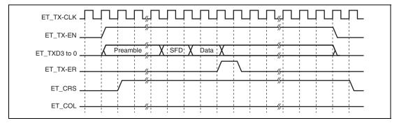
Figure 23.19 MII Frame Transmit Timing (Transmit Error)
