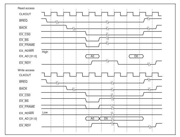
Figure 15.2 External CPU Access (Single Access)
