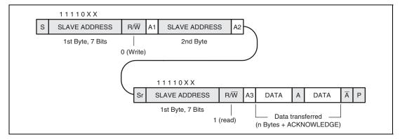
Figure 26.7 10-Bit Address Data Receive Format
