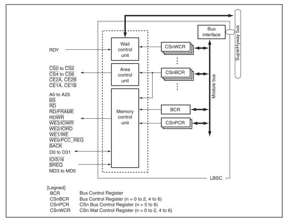
Figure 11.1 LBSC Block Diagram
