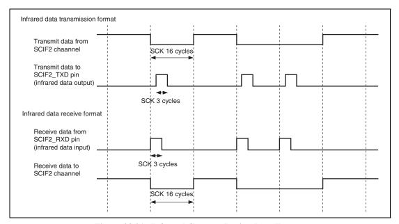
Figure 28.21 Infrared Communication Data Format
