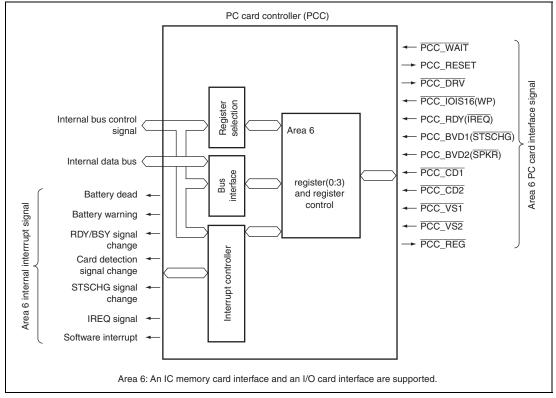
Figure 32.1 PC Card Controller Block Diagram
