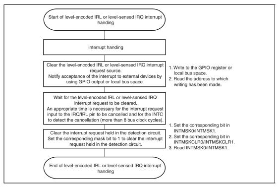
Figure 9.5 Example of Interrupt Handling Routine
