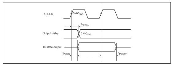
Figure 43.35 Output Signal Timing
