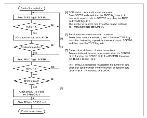
Figure 28.7 Sample Serial Transmission Flowchart
