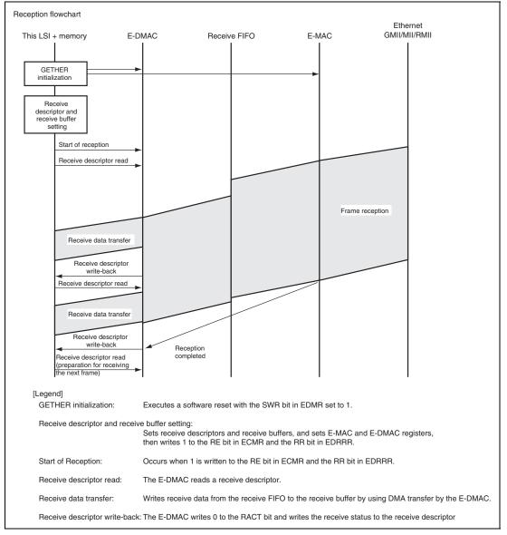
Figure 23.11 Sample Reception Flowchart (Single-Frame/Two-Descriptor)
