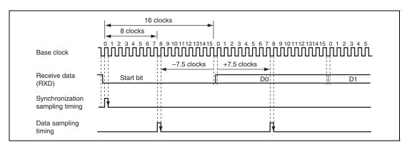
Figure 28.20 Receive Data Sampling Timing in Asynchronous Mode
