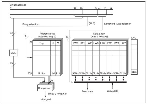
Figure 7.1 Configuration of Operand Cache (OC)
