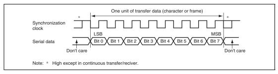
Figure 28.12 Data Format in Clocked Synchronous Communication
