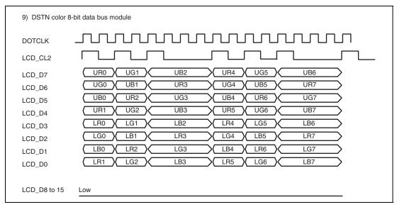
Figure 37.19 Clock and LCD Data Signal Example (DSTN Color 8-Bit Data Bus Module)
