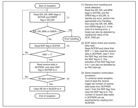
Figure 27.12 Sample Serial Reception Flowchart (1)
