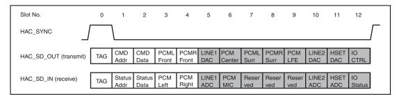
Figure 33.2 AC97 Frame Slot Structure
