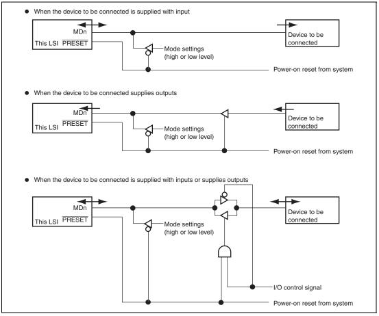
Figure B.1 Schematic Diagram of External Circuits
