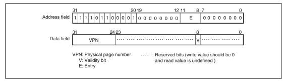
Figure 6.18 Memory-Mapped PMB Address Array
