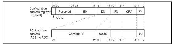
Figure 13.15 Address Generation for Type 0 Configuration Access
