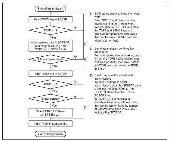
Figure 27.9 Sample Serial Transmission Flowchart
