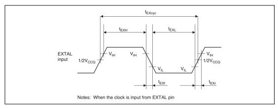
Figure 43.2 EXTAL Clock Input Timing
