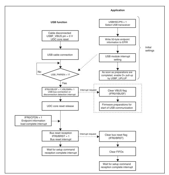
Figure 36.3 Cable Connection Operation
