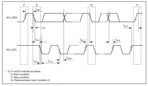
Figure 43.56 I<sup>2</sup>C Bus Interface Input/Output Timing
