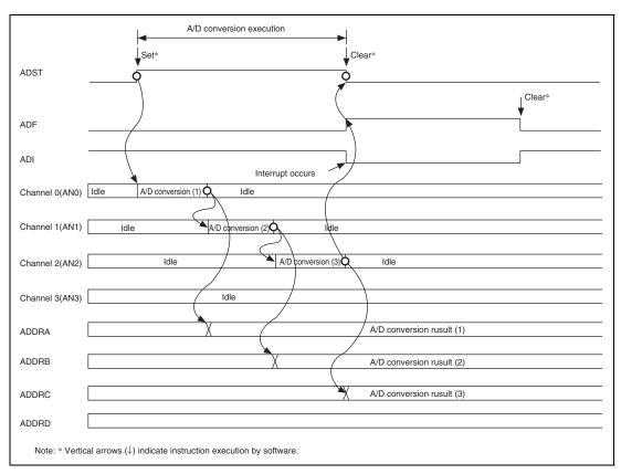
Figure 38.3 Example of A/D Converter Operation (Multi Mode, Three Channels AN0 to AN2 Selected)
