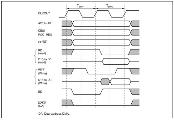
Figure 11.17 Basic Timing for PCMCIA Memory Card Interface
