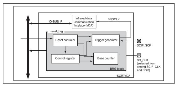
Figure 28.23 BRG Block Diagram
