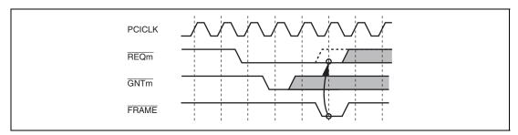
Figure 13.27 Timing Example of Device (REQm) Not Executing REQ Negation and FRAME
