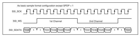
Figure 34.12 Inverted Padding Polarity
