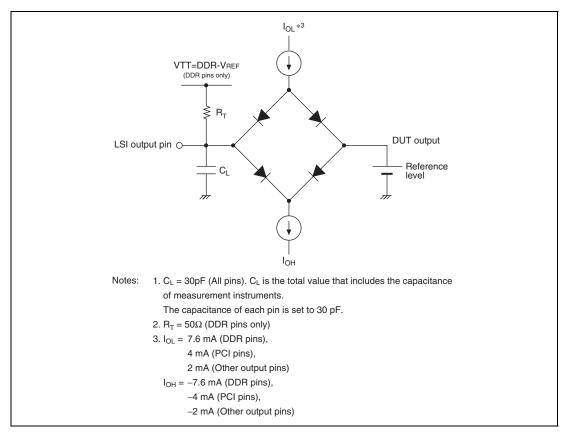
Figure 43.85 Output Load Circuit
