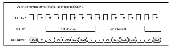
Figure 34.10 Inverted Clock
