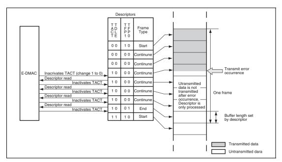
Figure 23.12 E-DMAC Operation after Transmit Error
