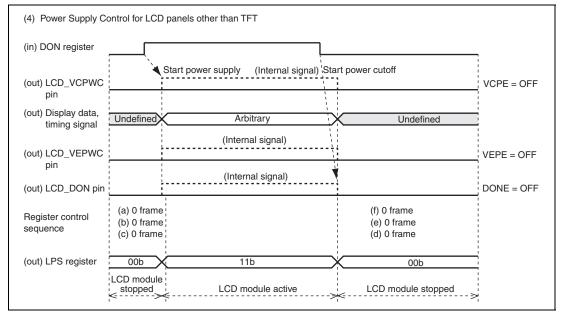
Figure 37.8 Power-Supply Control Sequence and States of the LCD Module
