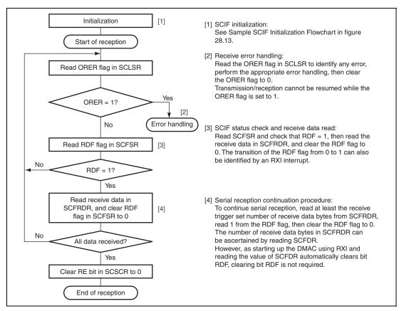
Figure 28.16 Sample Serial Reception Flowchart (1)
