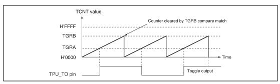
Figure 20.7 Example of Toggle Output Operation
