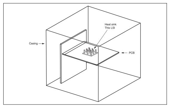
Figure H.1 Overall View of Simulation Model (with heat sink)
