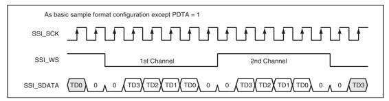
Figure 34.16 Parallel Right Aligned with Delay
