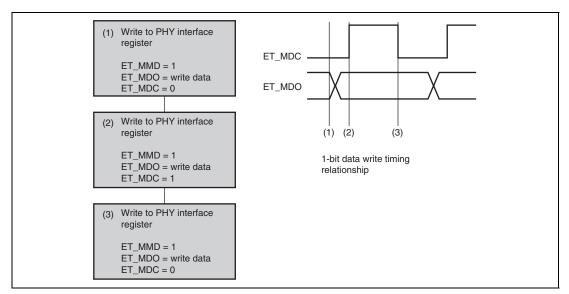
Figure 23.33 1-Bit Data Write Flowchart
