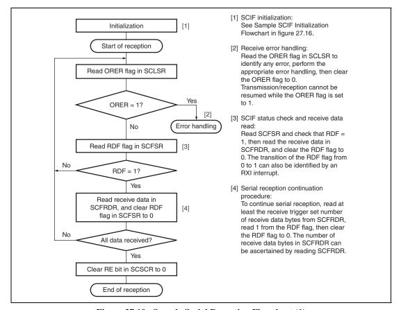
Figure 27.19 Sample Serial Reception Flowchart (1)
