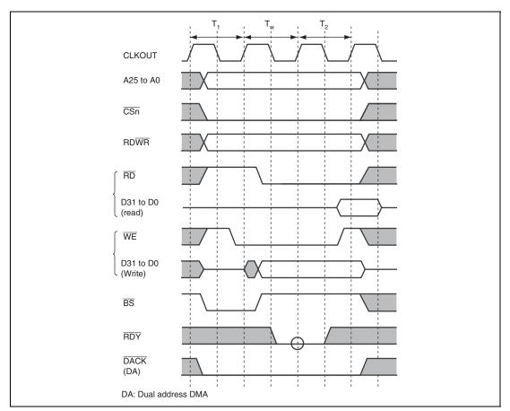
Figure 11.9 SRAM Interface Wait Timing (Software Wait Only)
