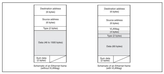
Figure 23.39 Data after Checksum Data Addition
