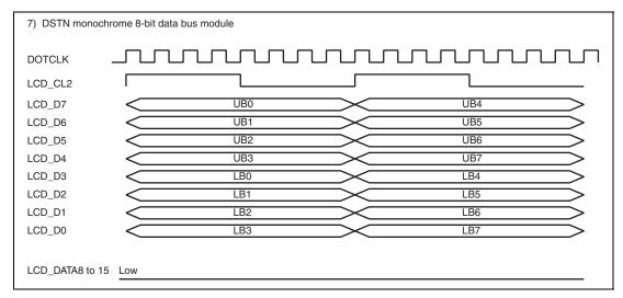
Figure 37.17 Clock and LCD Data Signal Example (DSTN Monochrome 8-Bit Data Bus Module)
