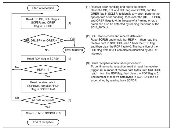
Figure 28.9 Sample Serial Reception Flowchart (1)
