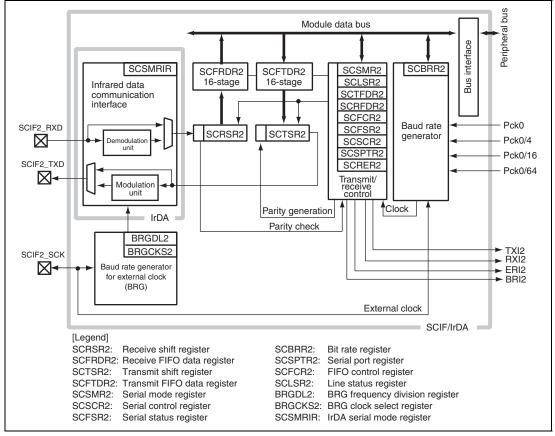
Figure 28.1 Block Diagram of SCIF/IrDA
