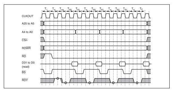
Figure 11.13 Burst ROM Wait Access Timing
