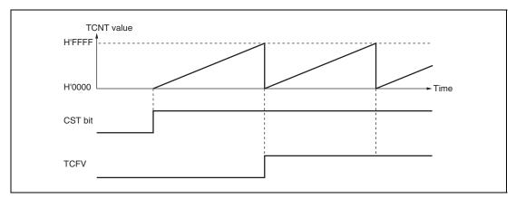
Figure 20.3 Free-Running Counter Operation
