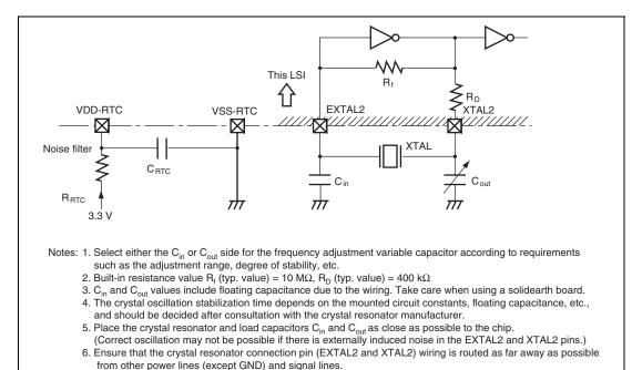
Figure 22.5 Example of Crystal Oscillator Circuit Connection
