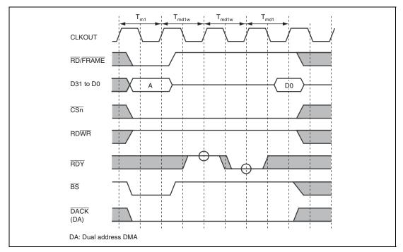
Figure 11.24 MPX Interface Timing 2 (Single Read, IW = 0, One External Wait Inserted)
