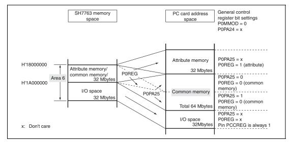
Figure 32.2 Continuous 32-Mbyte Area Mode
