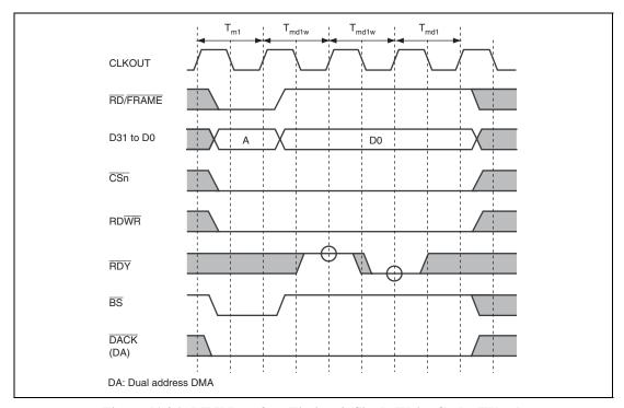
Figure 11.26 MPX Interface Timing 4 (Single Write Cycle, IW = 1, One External Wait Inserted)
