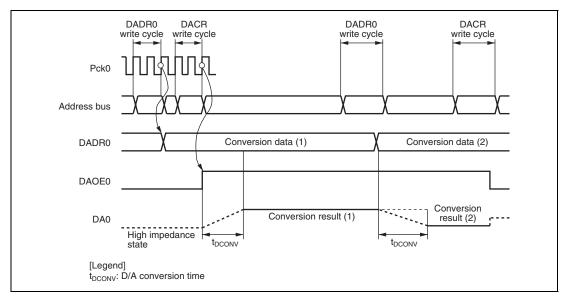
Figure 39.2 D/A Converter Operation Example
