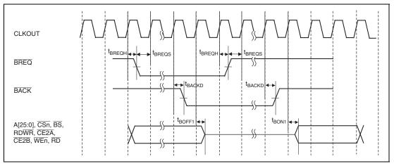
Figure 43.9 Control Signal Timing
