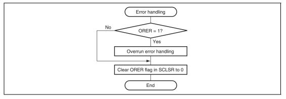
Figure 28.17 Sample Serial Reception Flowchart (2)
