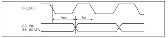
Figure 43.77 SSI Receive Timing (2)
