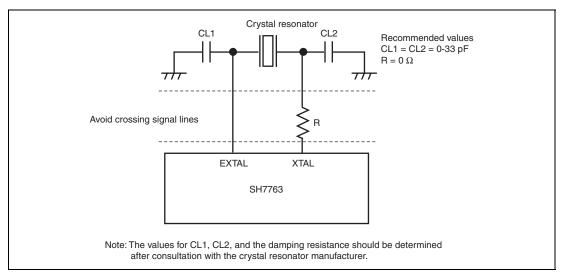
Figure 16.2 Notes on Using Crystal Resonator
