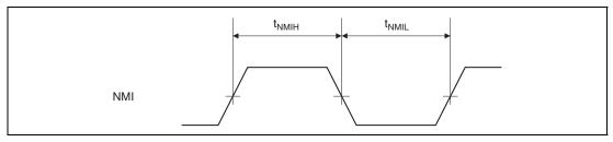
Figure 43.31 NMI Input Timing
