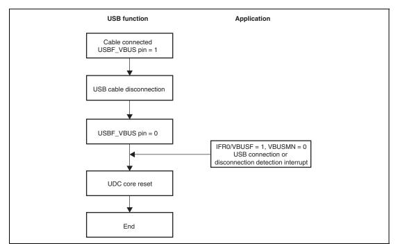
Figure 36.4 Cable Disconnection Operation
