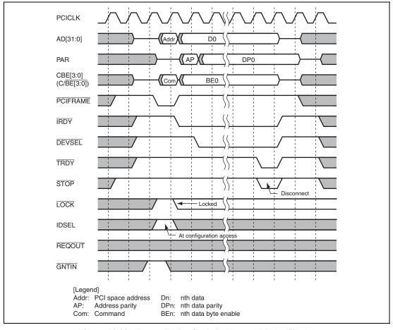
Figure 13.22 Target Write Cycle in Normal Mode (Single)
