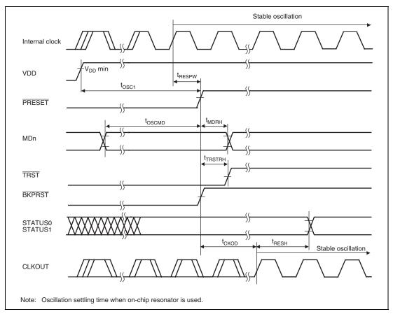
Figure 43.5 Power-On Oscillation Settling Time
