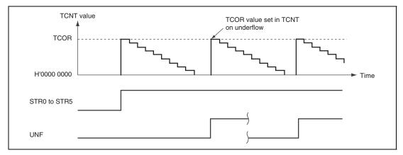
Figure 19.3 TCNT Auto-Reload Operation
