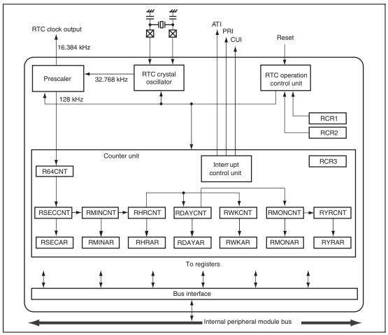
Figure 22.1 Block Diagram of RTC
