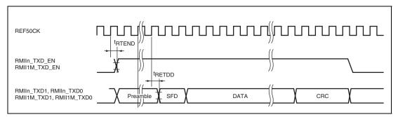
Figure 43.49 RMII Transmit Timing
