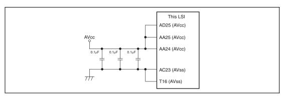
Figure C.1 Connection Example of Bypass Capacitors for Analog Power Supply
