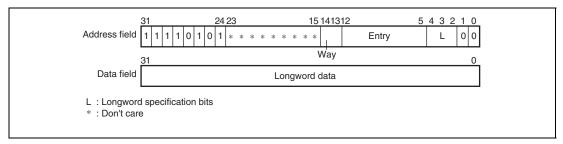
Figure 7.8 Memory-Mapped OC Data Array
