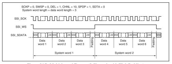
Figure 34.7 Multichannel Format (3 Channels with High Padding)
