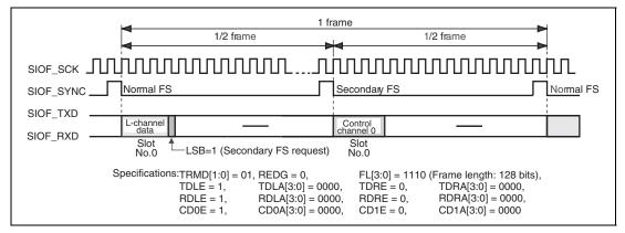
Figure 29.8 Control Data Interface (Secondary FS)
