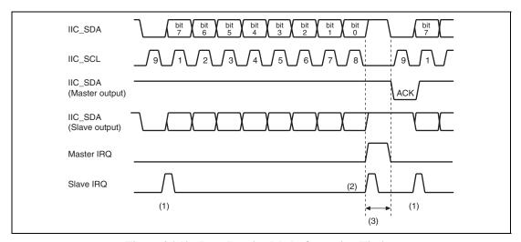
Figure 26.10 Data Receive Mode Operation Timing
