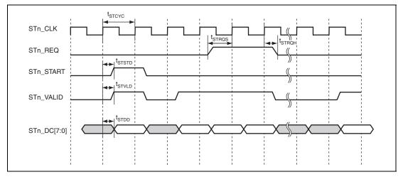
Figure 43.53 STIF Clock Valid Transmit Timing
