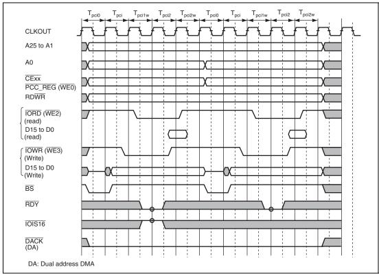
Figure 11.21 Dynamic Bus Sizing Timing for PCMCIA I/O Card Interface
