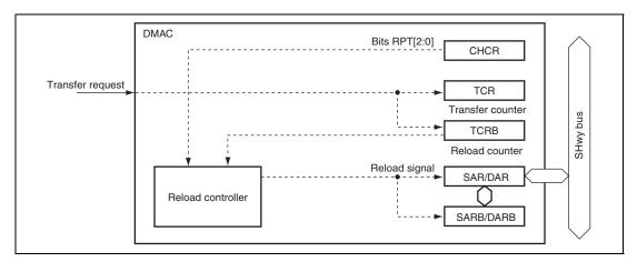
Figure 14.12 Reload Mode Transfer
