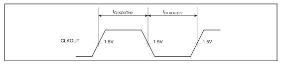
Figure 43.4 CLKOUT Clock Output Timing (2)
