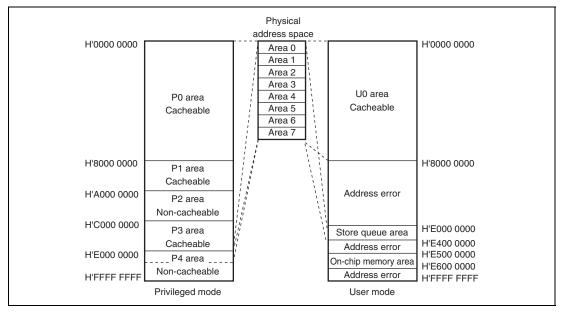
Figure 6.2 Virtual Address Space (AT in MMUCR = 0)
