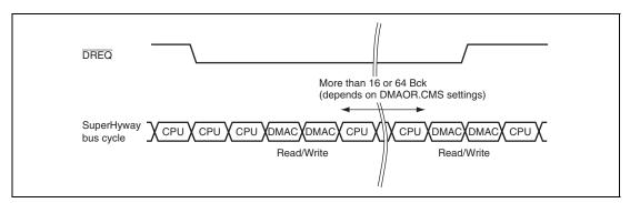
Figure 14.8 Example of DMA Transfer Timing in Cycle Steal Intermittent Mode (DREQ Low Level Detection)
