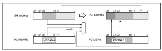
Figure 13.3 SuperHyway Bus to PCI Local Bus Address Translation (PCI Memory Space 0)
