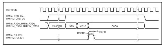
Figure 43.51 RMII Receive Timing (When an Error is Detected)
