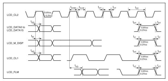
Figure 43.79 LCDC Module Signal Timing
