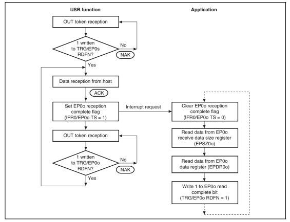
Figure 36.7 Data Stage (Control-Out) Operation
