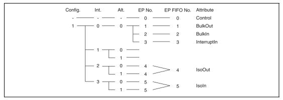
Figure 36.2 Example of Endpoint Configuration
