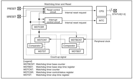
Figure 17.1 System Block Diagram
