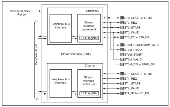
Figure 25.1 Block Diagram of STIF
