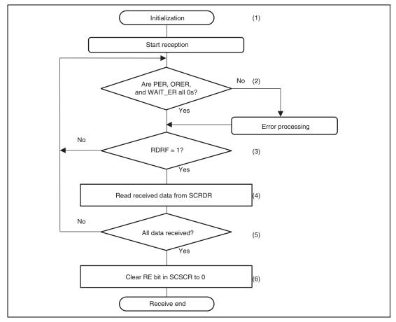
Figure 30.6 Example of Receive Processing
