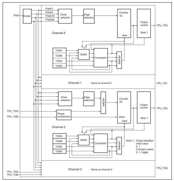
Figure 20.1 Block Diagram of TPU
