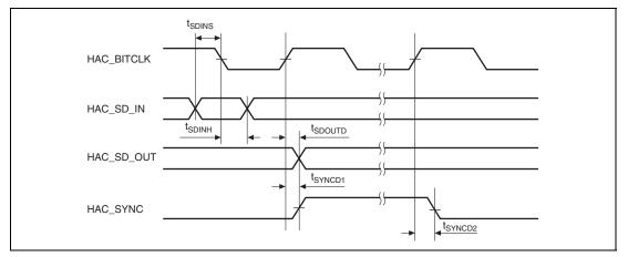
Figure 43.72 HAC Interface Module Signal Timing
