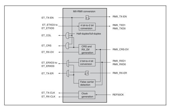
Figure 23.37 MII-RMII Conversion Circuit
