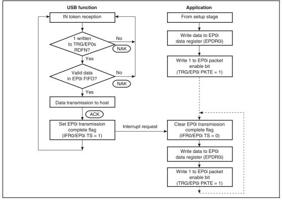
Figure 36.6 Data Stage (Control-In) Operation
