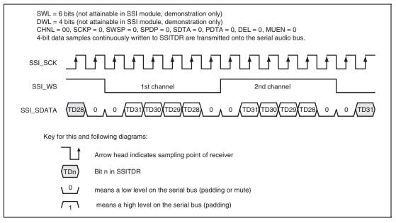
Figure 34.9 Basic Sample Format (Transmit Mode with Example System/Data Word Length)
