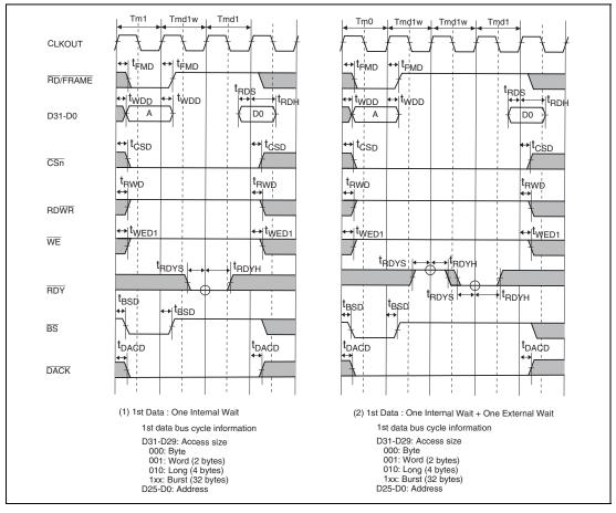
Figure 43.22 MPX Basic Bus Cycle: Read
