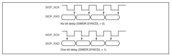
Figure 29.21 SIOF Receive Data Sampling Timing in Slave Mode
