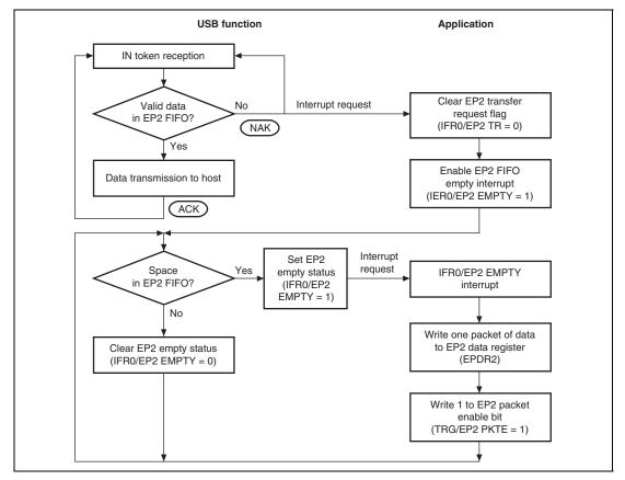
Figure 36.11 EP2 Bulk-In Transfer Operation
