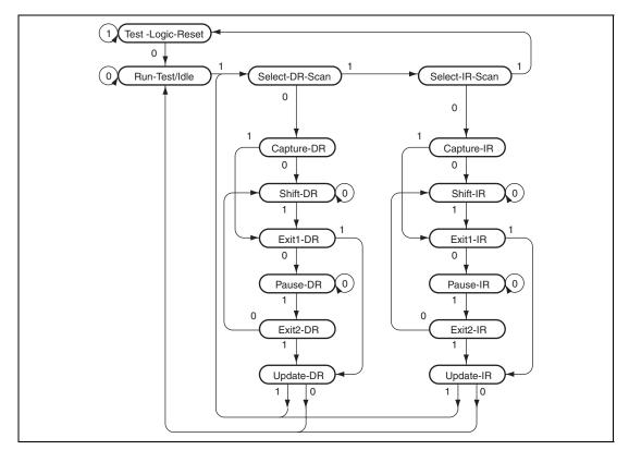
Figure 42.3 TAP Controller State Transitions
