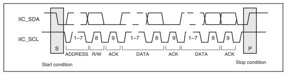
Figure 26.2 I<sup>2</sup>C Bus Timing
