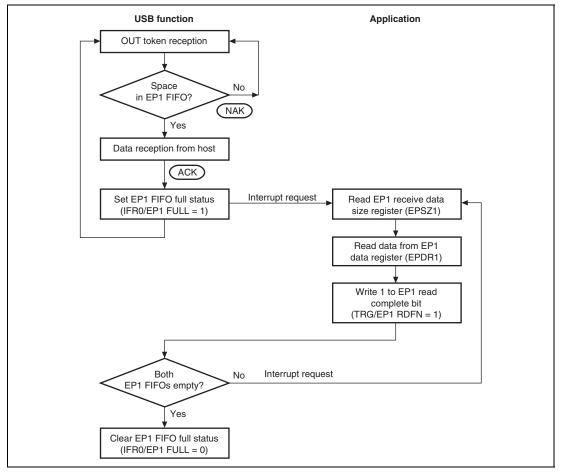
Figure 36.10 EP1 Bulk-Out Transfer Operation
