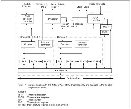
Figure 19.1 Block Diagram of TMU
