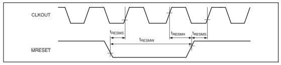
Figure 43.8 Reset Input Timing
