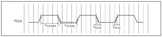
Figure 43.38 TCLK Input Timing
