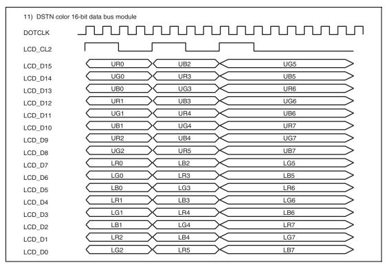
Figure 37.21 Clock and LCD Data Signal Example (DSTN Color 16-Bit Data Bus Module)
