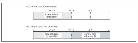
Figure 29.6 Control Data Bit Alignment
