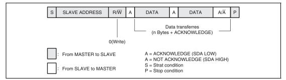
Figure 26.3 Master Data Transmit Format
