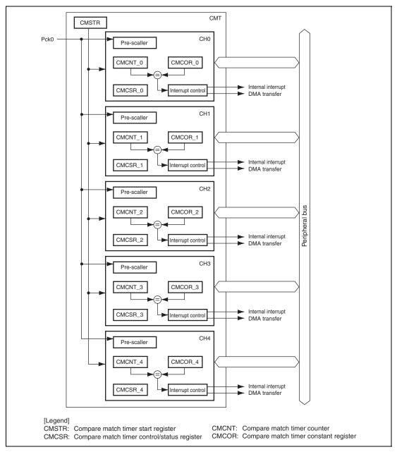
Figure 21.1 Block Diagram of CMT
