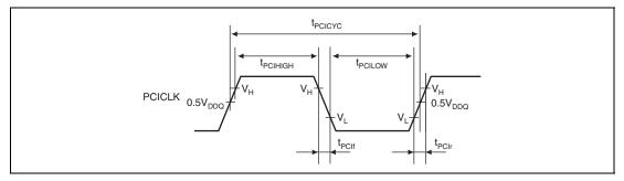
Figure 43.34 PCI Clock Input Timing
