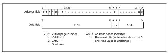
Figure 6.12 Memory-Mapped ITLB Address Array
