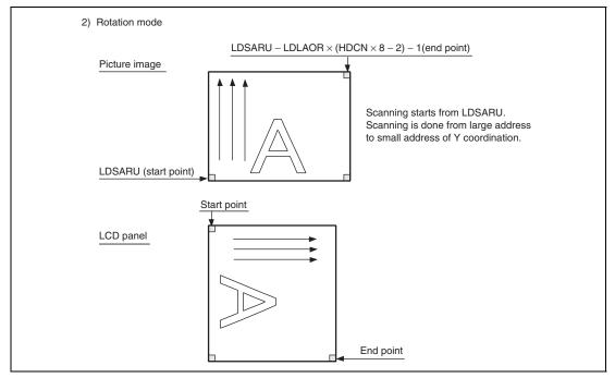
Figure 37.10 Operation for Hardware Rotation (Rotation Mode)
