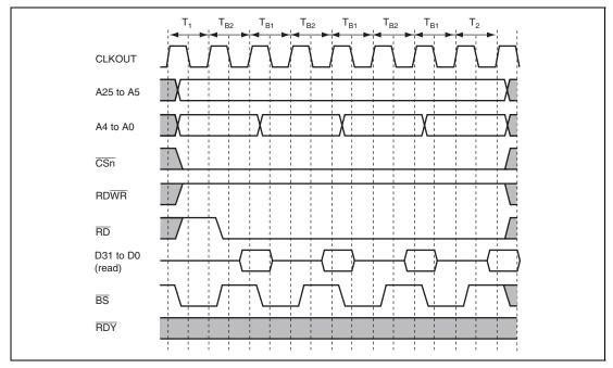
Figure 11.12 Burst ROM Basic Access Timing
