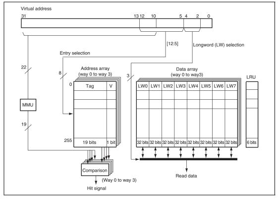
Figure 7.2 Configuration of Instruction Cache (IC)
