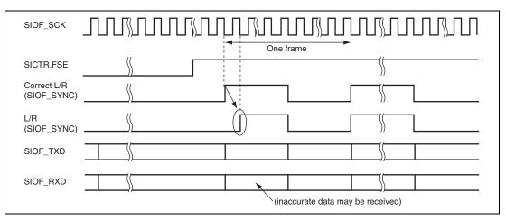
Figure 29.23 SIOF\_SYNC Output Timing in Master Mode 2 (Transfer Resumed)
