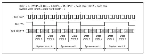
Figure 34.6 Multichannel Format (2 Channels, No Padding)
