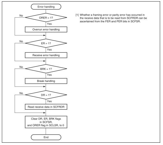
Figure 28.10 Sample Serial Reception Flowchart (2)
