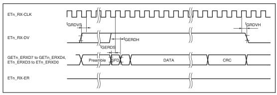
Figure 43.46 GMII Receive Timing (normal operation)
