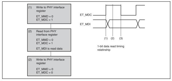
Figure 23.35 1-Bit Data Read Flowchart
