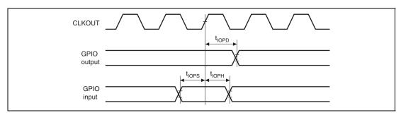
Figure 43.80 GPIO Timing
