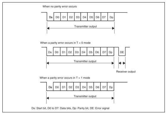
Figure 30.2 Data Format Used by Smart Card Interface
