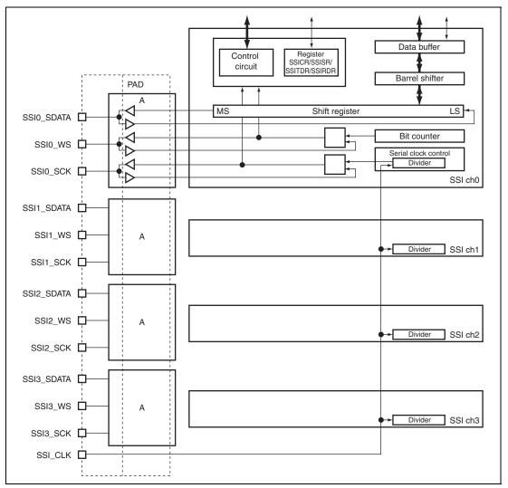
Figure 34.1 Block Diagram of SSI Module
