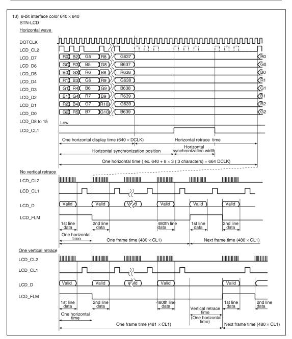
Figure 37.23 Clock and LCD Data Signal Example (8-Bit Interface Color  $640 \times 480$ )
