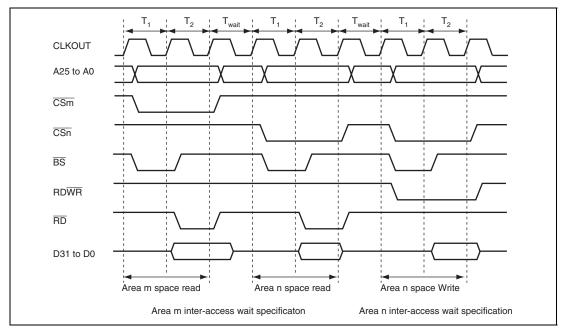
Figure 11.39 Wait Cycles between Access Cycles
