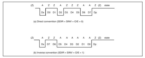
Figure 30.3 Examples of Start Character Waveforms
