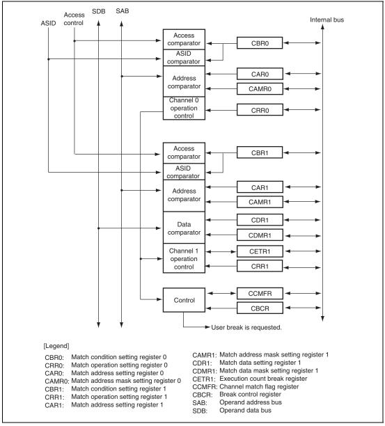
Figure 41.1 Block Diagram of UBC
