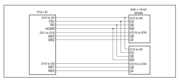
Figure 11.35 Example of 32-Bit Data-Width Byte-Control SRAM
