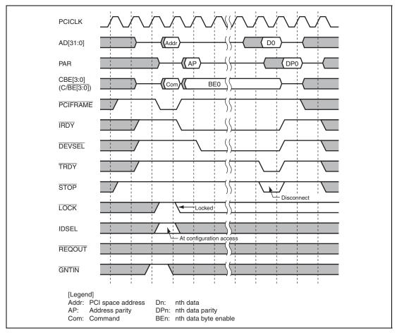
Figure 13.21 Target Read Cycle in Normal Mode (Single)
