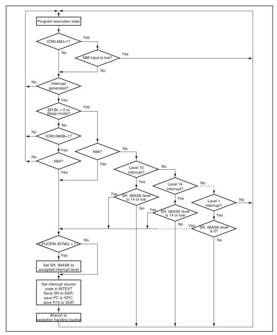
Figure 9.4 Interrupt Operation Flowchart
