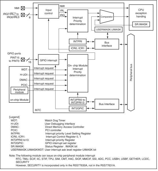
Figure 9.1 Block Diagram of INTC
