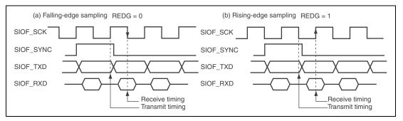
Figure 29.4 SIOF Transmit/Receive Timing
