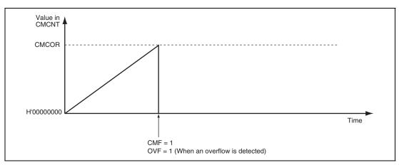
Figure 21.2 Counter Operation (One-Shot Operation)
