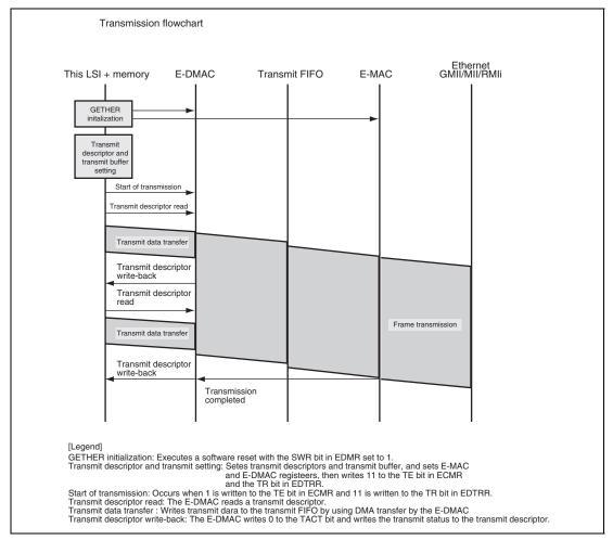
Figure 23.8 Sample Transmission Flowchart (Single-Frame/Two-Description)
