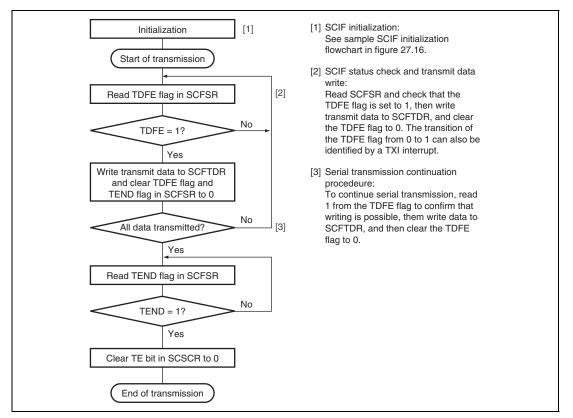
Figure 27.17 Sample Serial Transmission Flowchart
