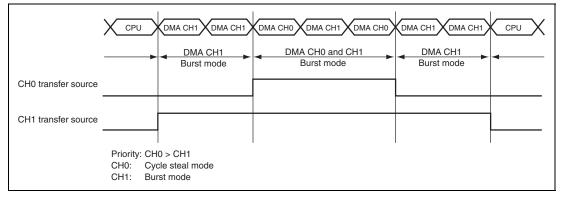
Figure 14.10 Bus State when Multiple Channels are Operating
