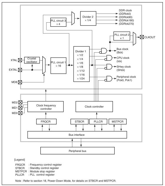
Figure 16.1 Block Diagram of CPG
