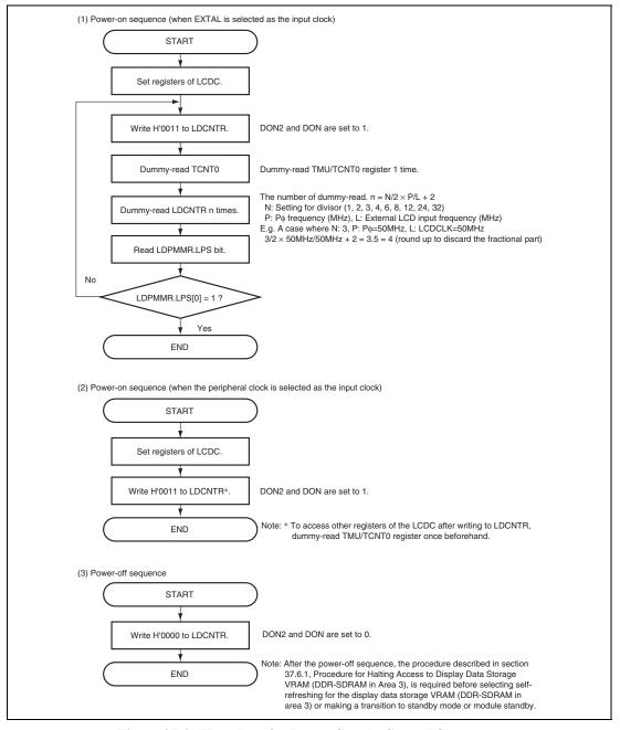
Figure 37.4 Flowchart for Power-Supply Control Sequences
