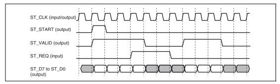
Figure 25.5 Clock Valid Transmission Timing
