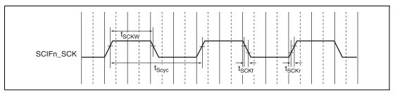
Figure 43.58 SCIFn\_SCK Input Clock Timing
