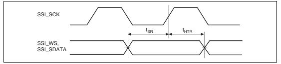
Figure 43.76 SSI Receive Timing (1)
