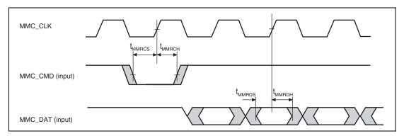
Figure 43.68 MMCIF Receive Timing (Sampling at the Rising Edge)
