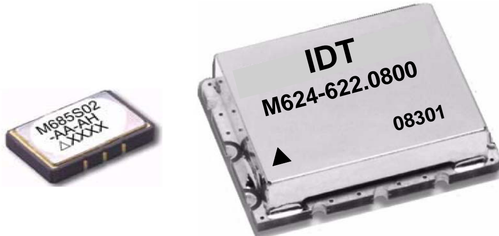
Figure 9 IDT 5x7mm Integrated Circuit VCSO and 15x20mm Discrete VCSO
