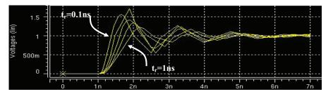
Having the ability to fine tune the rise/fall time via pins or a programmable interface opens up a new level of control to create and maintain quality signals. The new family of IDT programmable clocks, starting with the 5V9885 (programmable generator), is leading the industry in enabling techniques that allow system engineers to optimize their designs for high signal fidelity.
