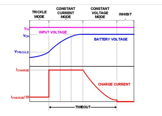
Figure 1. A typical charging curve for a lithium battery.
