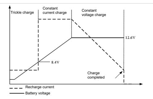
Figure 2. Charge current and voltage.
