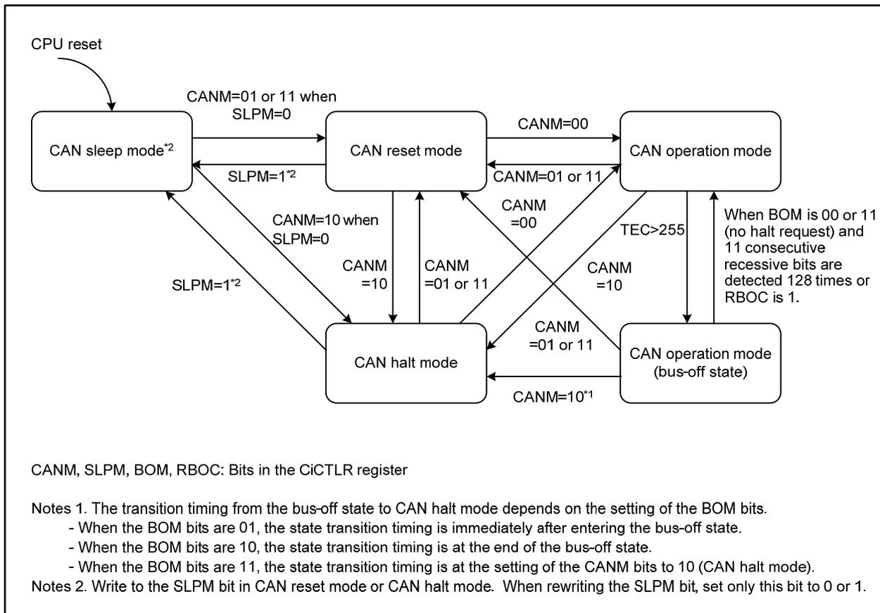
Figure 20.9 Transition between CAN Operating Modes (i=0 to 5)
