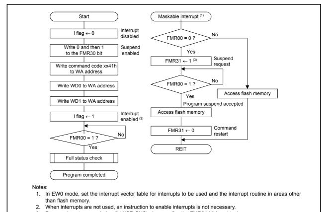
3. Program is not suspended until td(SR-SUS) elapses after the FMR31 bit is set to 1.
