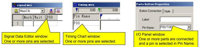
In addition, if connection pins are added or deleted in the Signal Data Editor window during program execution, the simulator may deadlock or may be forcibly terminated.
