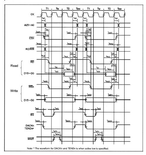
Figure 27.15 Basic Bus Timing for Normal Space
