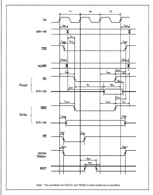
Figure 27.13 Basic Bus Timing for Normal Space (One Software Wait Cycle)
