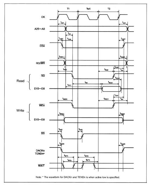
Figure 27.14 Basic Bus Timing for Normal Space (One External Wait Cycle)
