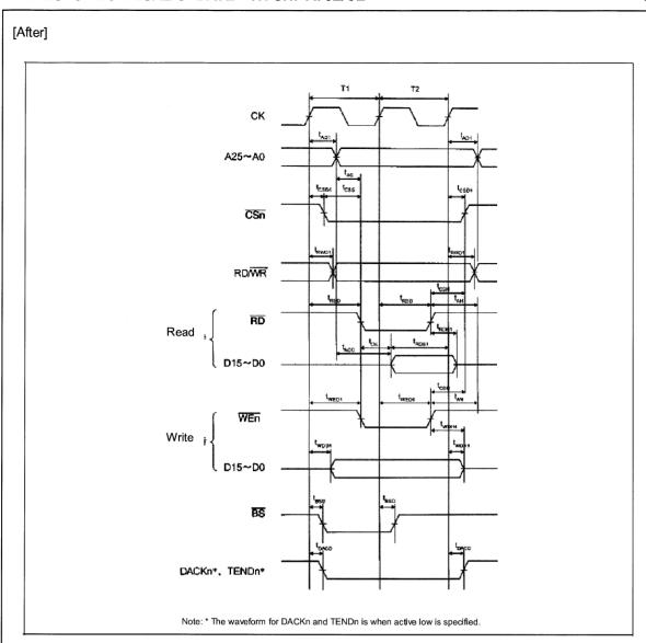
Figure 27.12 Basic Bus Timing for Normal Space (No Wait)
