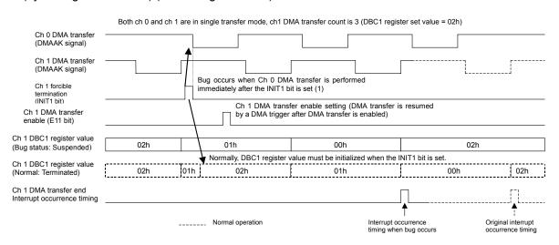
This bug does not depend on the number of transfer channels, transfer type (2-cycle or flyby), transfer target (between memory and memory, memory and I/O; including internal resources), transfer mode (single, single-step, or block), or trigger (external request, interrupt from internal
