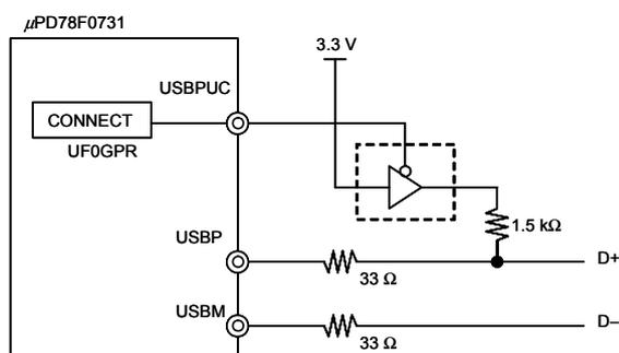
Figure 3-2. Circuit in IECUBE (Before Change)
