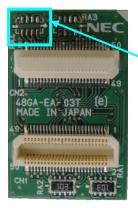
Module resistors have been removed.
