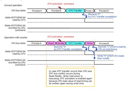
Figure 2. condition of CPU bus and DTC Activation Enable Register
