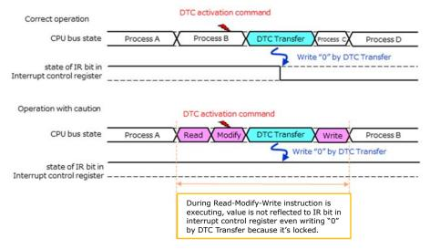
Figure 1. condition of CPU bus and interrupt control register
