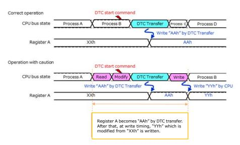
Figure 3. Condition of CPU bus and specific register
