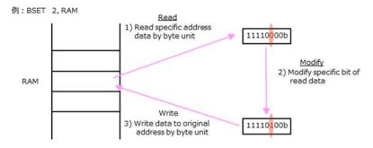
Figure 4. operation of Read-Modify-Write instruction
