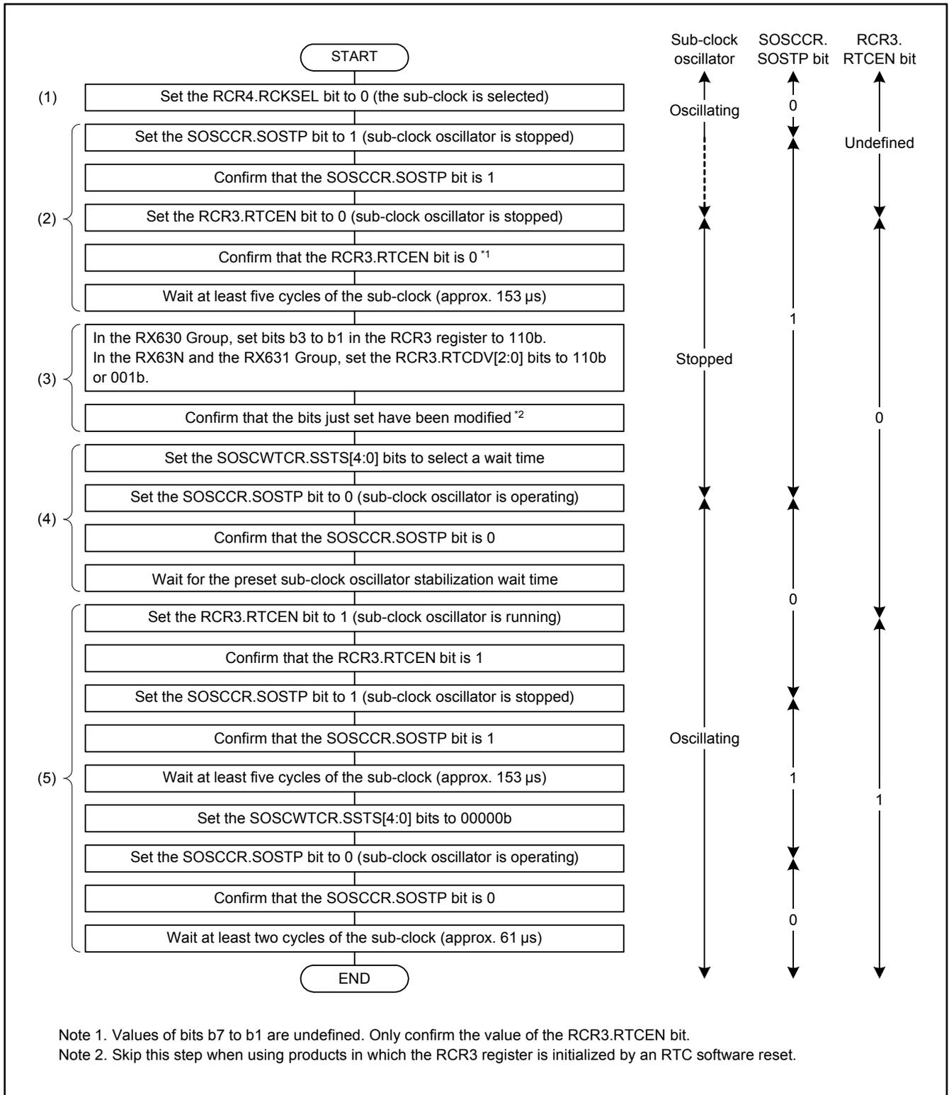
Figure 2.1 Initialization Flowchart When Using the Sub-clock as an RTC Count Source
