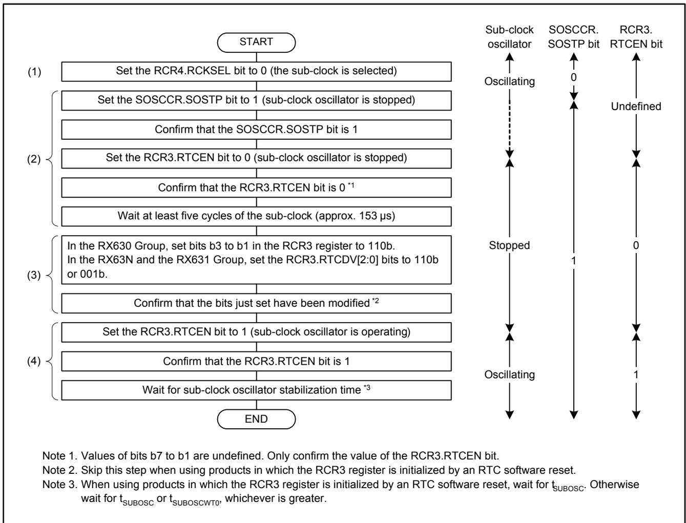
**Figure 2.2 Initialization Flowchart When Using the Sub-clock Only as an RTC Count Source**
