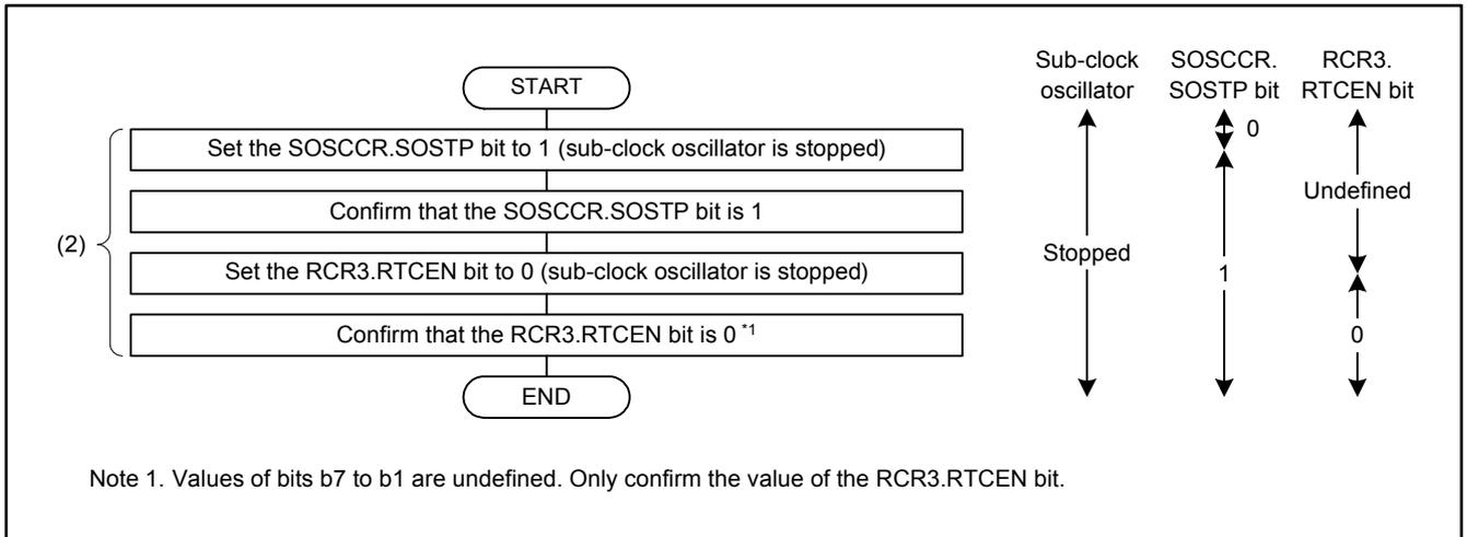
**Figure 2.4 Initialization Flowchart When Not Using the Sub-clock**
