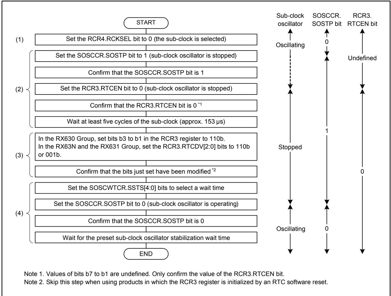
**Figure 2.3 Initialization Flowchart When Using the Sub-clock Only as a System Clock**
