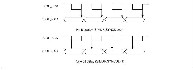
Figure. SIOF Receive Data Sampling Timing in Slave Mode
