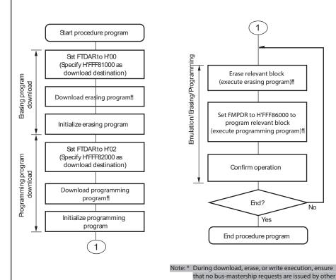
Figure 21.13 Sample Procedure of Repeating RAM Emulation, Erasing, and Programming (Overview)
