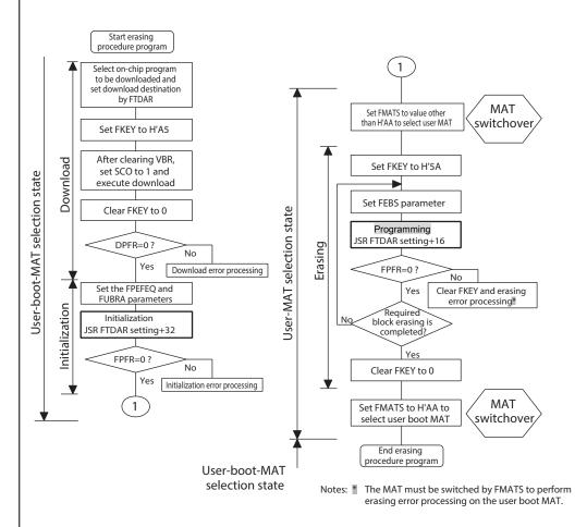
Figure 21.15 Procedure for Erasing User MAT in User Boot Mode
