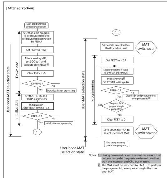
Figure 21.14 Procedure for Programming User MAT in User Boot Mode
