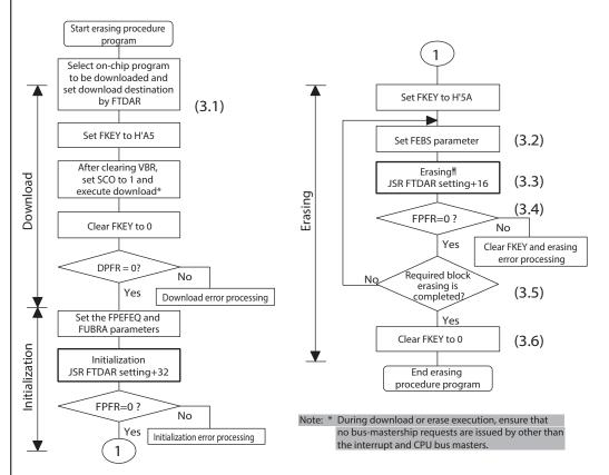
Figure 21.12 Erasing Procedure
