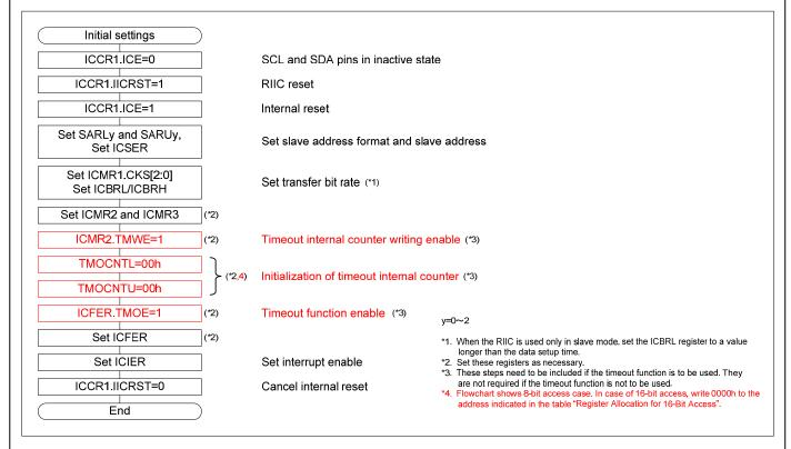
Figure 29.5 Example of RIIC Initialization Flow
