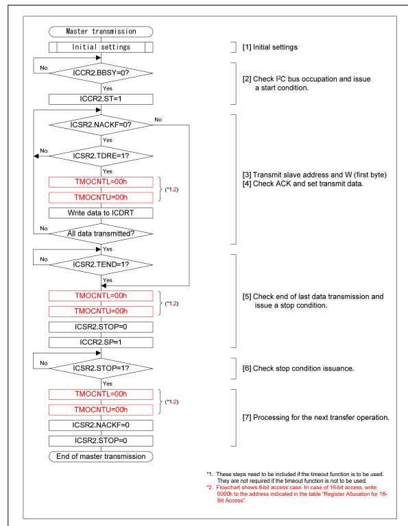
Figure 29.6 Example of Master Transmission Flowchart
