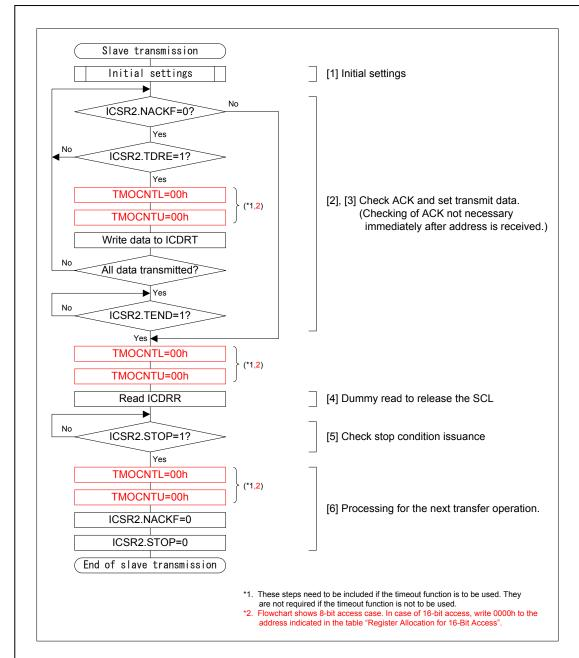
Figure 29.14 Example of Slave Transmission Flowchart
