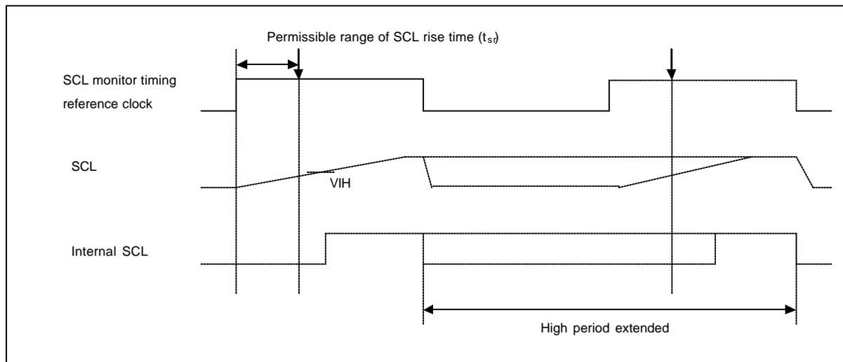
Figure 1 Bit Synchronization Circuit Timing
