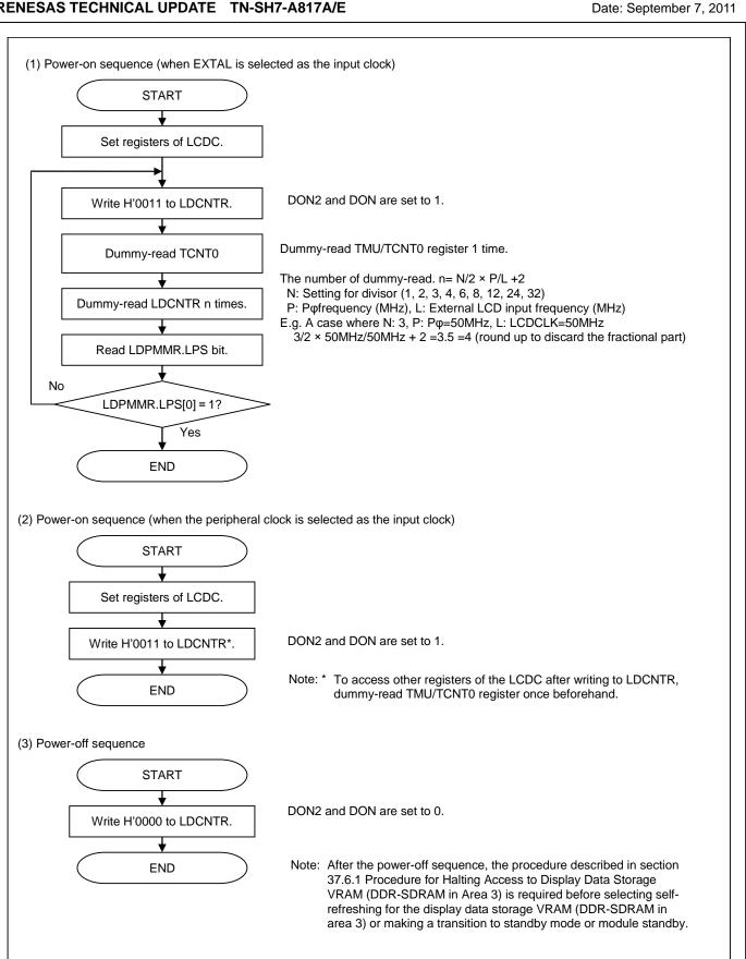
Figure 37.4 Flowchart for Power-Supply Control Sequences
