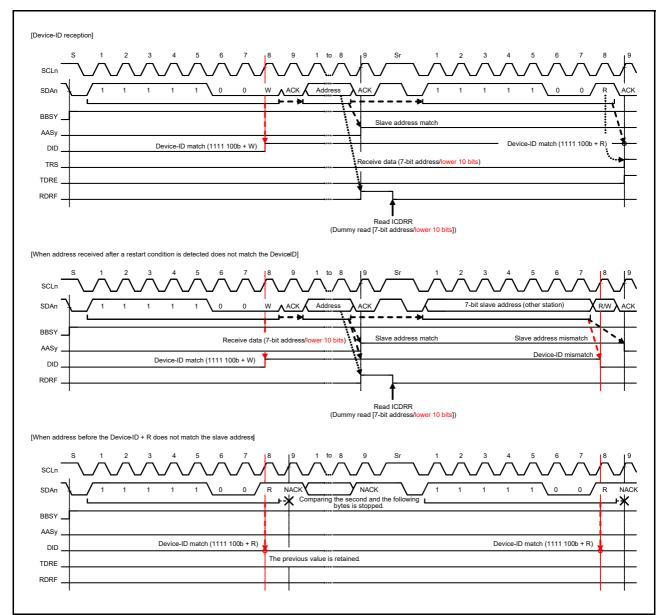
Figure 33.28 AASy/DID Flag Set/Clear Timing during Reception of Device-ID
