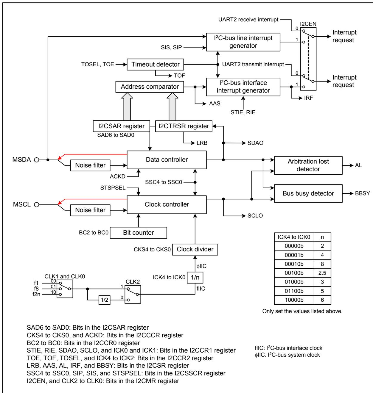
**Figure 24.1 Multi-master I<sup>2</sup>C-bus Interface Block Diagram**
