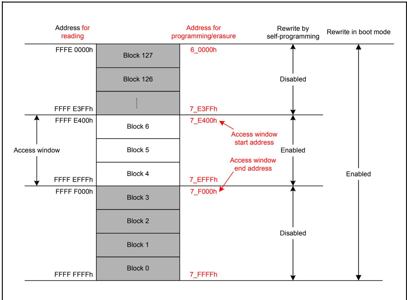
Figure 35.4 Area Protection Overview (Set Blocks 4 to 6 as the Access Window)
