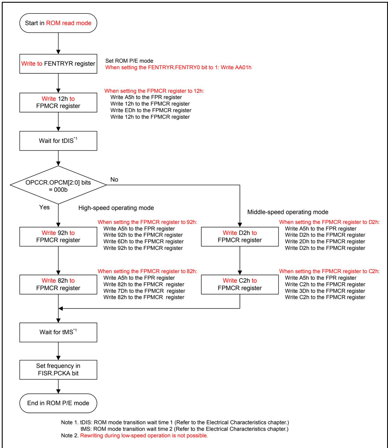
**Figure 35.6 Procedure for Transition to ROM P/E Mode**
