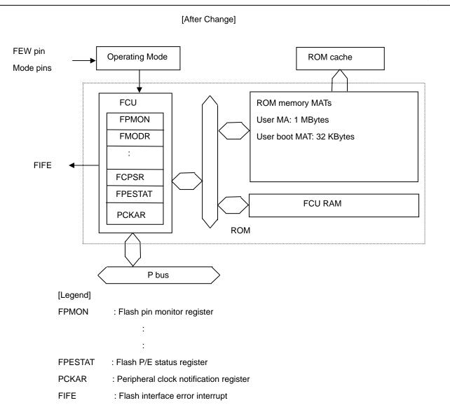
Figure 27.2 Block Diagram of ROM
