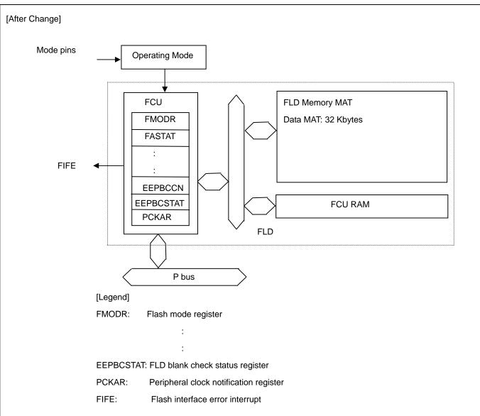
Figure 28.2 Block Diagram of FLD
