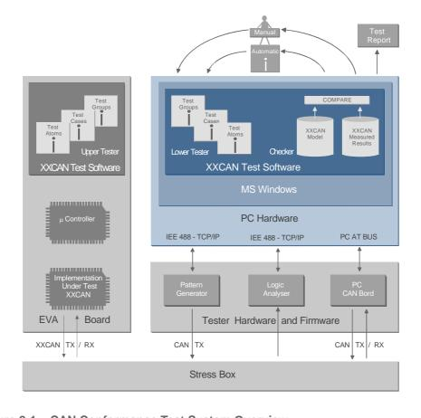
Figure 2-1 CAN Conformance Test System Overview
