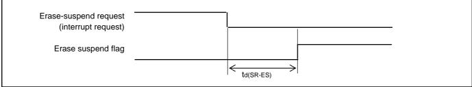
Figure 1 Time delay from suspend request until erase suspend
