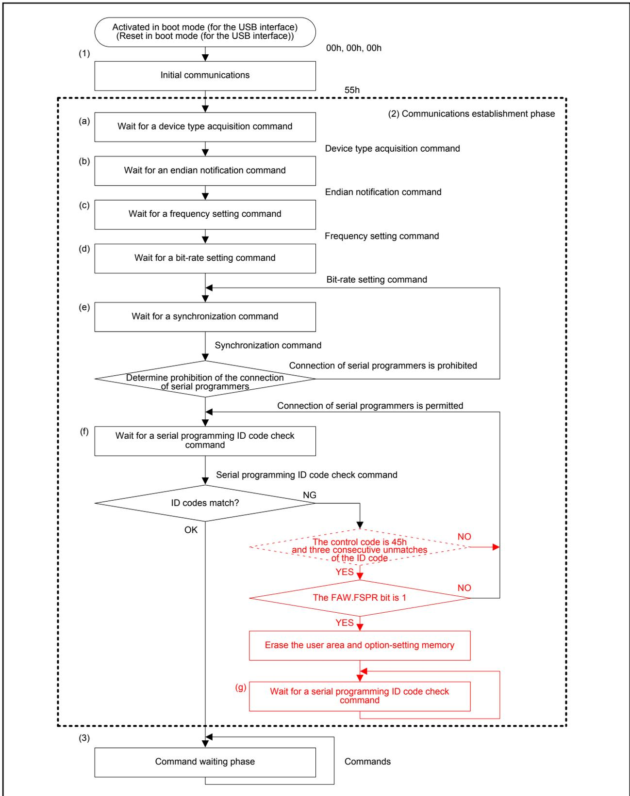
Figure 56.9 State Transition Flow in Boot Mode (for the USB Interface)
