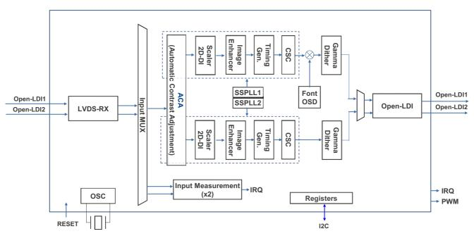
Figure 1. TW8849 Functional Block Diagram
