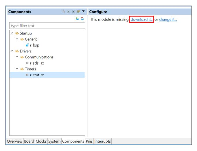
Figure 2-1: Download feature for missing FIT modules
