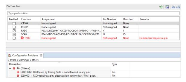
Figure 6-2: Ignore warnings when TXDn pin is disabled (Example with TXD0)
