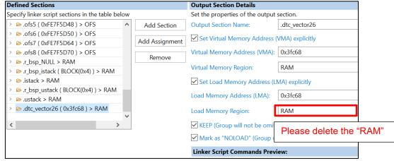
Figure 5-3: The workaround to resolve the section build issue
