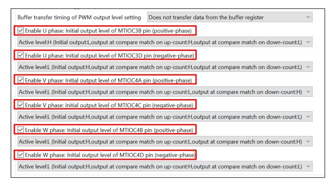
Figure 3-4: New check boxes for enabling/disabling the usage of U, V and W phase MTU pins
