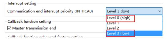
Figure 3-1 Priority level selection in components' UI
