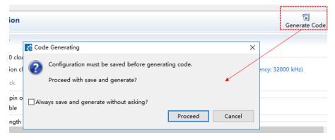
Figure 2-2 A warning dialog is added for reminding user to save the project
