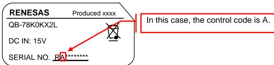
Figure 2. Checking Control Code for 'IECUBE Self Check Tool'
