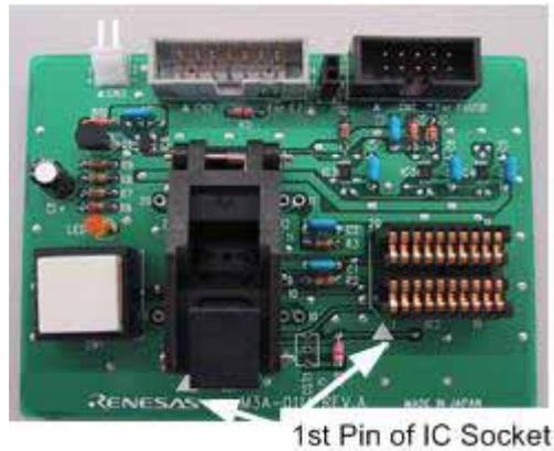
Procedure 1 Mount a MCU into the IC socket on the M3A-0114.
