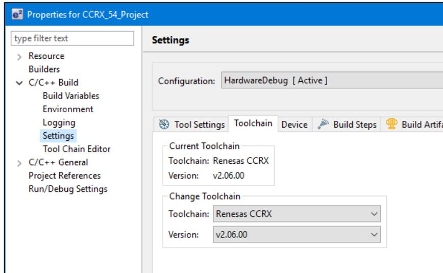
If the particular toolchain version does not exist and build is performed, then an error message is displayed and the build will fail.
