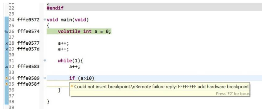
Hovering over the breakpoints which are not set will clearly show the reason for the failure.
