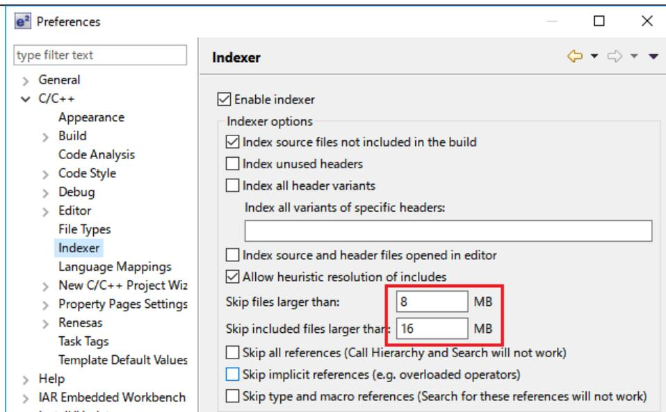
Put larger values for each red-framed variables, then rebuild project or rebuild index.
