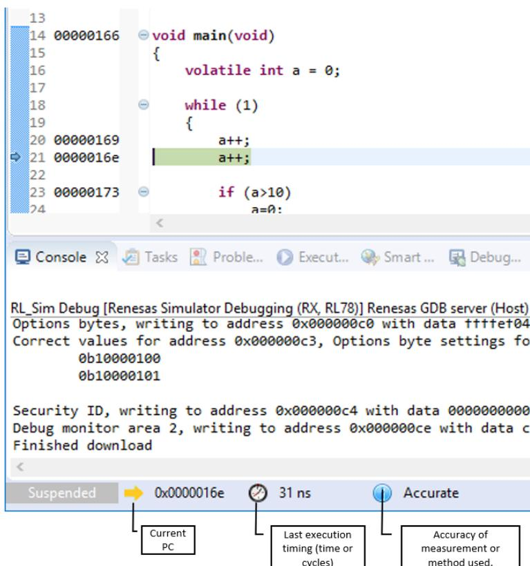
The view shows the current program counter (PC), the last execution timing either in time or CPU cycles and the accuracy or measurement method used.
