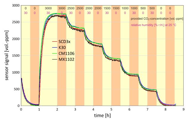
Fig. 10: Testing of IR-CO<sub>2</sub>-GS (MSS 4) in CO<sub>2</sub>-containing mixtures with different relative humidity
