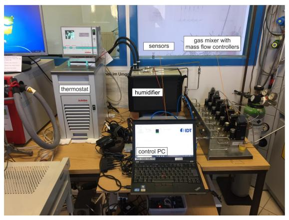
The humidifier for the synthetic air is a purpose-built arrangement of six horizontally positioned glass tubes that is described in detail earlier [3]. The home-build setup for preparation of the ethanol-mixture and its usage is described in detail in [4].
