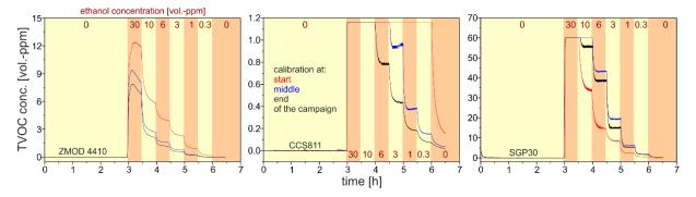
Fig. 6: e(CO<sub>2</sub>) values of MOX-GS (MSS 1) during ethanol calibrations; left: ZMOD 4410 No. x0000464045C23FBB, middle: CCS811 No. 005A558C, right: SGP30 No. 8478948
